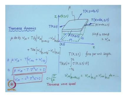
So, this must be the equation of, this must lead us to the equation of transverse dynamics. So, if you divide through out by dx dy and make some simplifications, so this, so del w/del x at x plus dx., so let me write this down. So, del w/del x(x+dx,y) may be written
