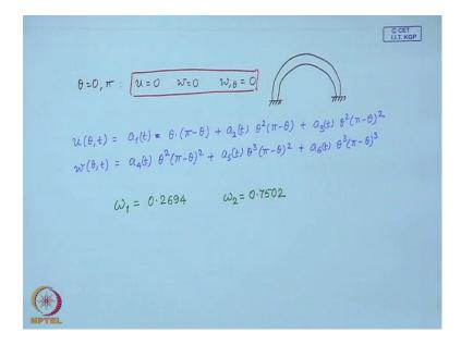
Now, in a similar manner you can perform for the clamped-clamped arch. So, this is the clamped-clamped arch. Here, the boundary conditions at zero and pi happen to be like this. Now, here all the boundary conditions are geometric boundary conditions.
