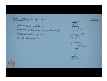
So, let us begin with axial vibrations of bars. So, where do we find bars in axial vibrations? So, some examples are in an ultrasonic machine. So, in an ultrasonic machine what you have is a bar, which is shaped like this, which is connected to an actuator. So, this bar is called a horn at the ultrasonic machine and this in ultrasonic generator which passes ultrasonic waves in this bar and because of the shape you have large amplitude
