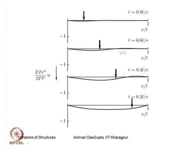
This figure shows the same thing when the speed is high. Now, here you can see a difference from the previous figure. In the previous figure, the deflection of the beam is completely on the negative side, below the equilibrium position. Now, here at certain time instant, this beam goes above the equilibrium line. Now, let us see this solution
