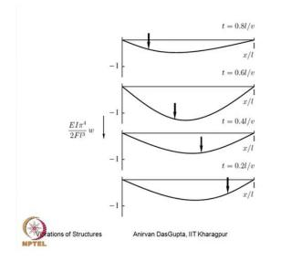
Now, let us look at this solution at certain time instant for two speeds, one is a low speed and other is a high speed transport over a beam. So, this figure shows snapshots at certain time instants for the force travelling on beam. So, you can see how the beam deflects at various time instants. Now, this is for low speed.
