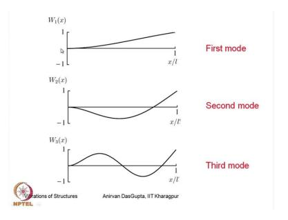
So, let us once look at these Eigen functions. So, this is the first mode, the first mode characterized by this Eigen function. This is the second mode; this is the third mode. So, you can see in the third mode there are two nodes; in the second mode there is only one node and no nodes in the first mode; and the slope here is zero, the displacement and slope as we expect.
