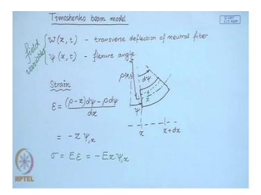
So, we are representing the slope of the neutral fiber in terms of this flexure angle and the shear strain. So, we can consider our field variables when we denote or represent the deflection of the beam, we can use any two of them. So, what we will do is, we will choose w and psi as our field variables.
