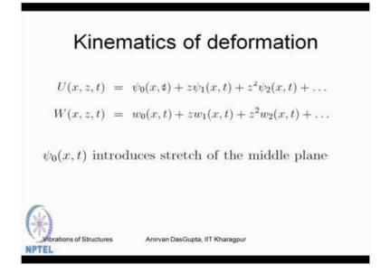
So, where capital U is the deflection in the axial direction; so it is being represented in terms of these functions psi 0, psi 1, psi 2, etc.; and expanded in terms of this variable z which is the location of this fiber from this point from the neutral axis. Similarly, this transverse deflection is also expanded as the series as powers of z, where we introduce these field variables  $w_0$ ,  $w_1$ ,  $w_2$ . Now, here this psi zero introduces the stretch of the middle plane.
