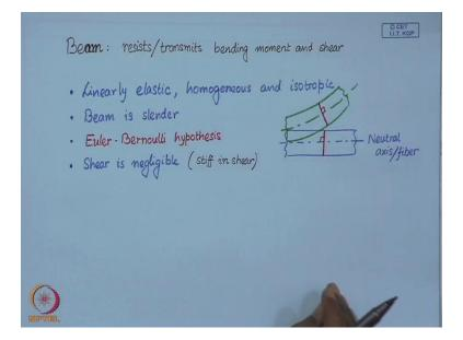
So, beam can resist or transmit bending moment and shear, and it is a one-dimensional elastic continuum. So, this is a distinctly different from the definition of a string, which cannot resist bending; and such examples we have seen in our previous lectures. Now
