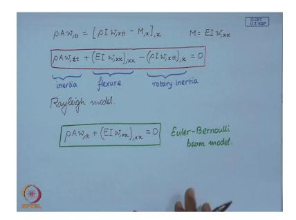
So, this was del V/del x. So, this is... and moment, the bending moment we have determined this... so therefore finally... So, if I rearrange this equation... so this is finally our equation of motion of the beam. Now here this term is known as the flexure term; this term is the rotary inertia term; and this is the normal transverse term or translation inertia term. So, this model of the beam is known as the Rayleigh model of the beam or Rayleigh beam model.
