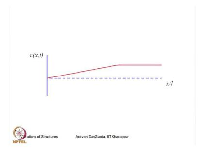
Now, here I have an animation, which shows the same thing. So, you can see this, so at this instant, now the propagation, now the compression wave is the propagating. So, this now in tension, on this side it is in compression, and this wave propagates back and forth in the bar, which is shown in the animation. Next, let us look at the another initial value problem, where we are going to have velocity initial condition.
