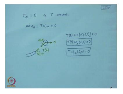
So, you can immediately see that the partial derivative of the tension in the string is 0; there is no external force in the in the longitudinal direction of the string. So, therefore, this is our equation for the tension, which implies the tension is a constant. So, if the
