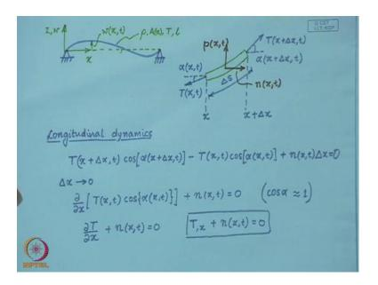
So, consider a string made of a material of density rho, has an area of cross section, which may be a function of the positional coordinate x; it is under a tension T and has the length l. So, this transverse motion of the string is measured by this variable w at a location x at a time instant t. So, so this shows a string, a stretched string or taut string, which has been displaced from its equilibrium position, which is the x axis. Now to write
