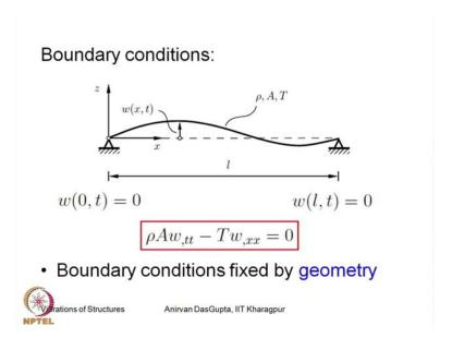
Now the boundary conditions now this is very simple. From geometry you can easily identify that at the left boundary and the right boundary, at both the boundaries, the displacement of the string must be 0. So, these boundary conditions are set by the geometry of the problem. So, the geometry of the problem says that the displacement, the transverse displacement of the string at the two boundaries must be 0. So these are the geometric boundary conditions for the string.
