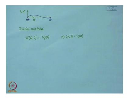
So, so as I mentioned that we need two initial conditions. So, these initial conditions are usually specified as the initial deformation of the string and the initial velocity distribution over the string. So, with these two initial conditions, one on the displacement, other on the velocity; we can now completely solve or uniquely solve the equation of motion of vibrating string. So, with this, we complete this part on the transverse vibrations of strings.
