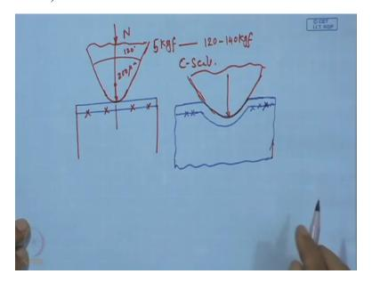
Now let us look how does it work, now say this is actually the coating and here we have the substrate, now on that this diamond brale of the Rockwell C-scale, so it is actually Rockwell c-scale that indenter and this is actually this diamond brale that means that it is a cone of diamond having a tip in the form of a hemisphere and this angle appears to be 120 degree.
