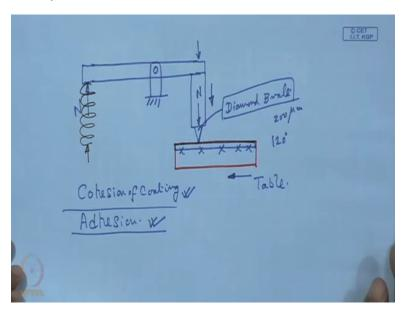
So what exactly we see here principle of scratch testing. Now in this principle of scratch testing what we see actually there is one arm, this is the apparatus, there is one arm which is pivoted at this point and then what we have here, we have one stylus and this is going to be an indenter, this is also a standardize that is also this Rockwell C-Scale, that means this diamond brale.
