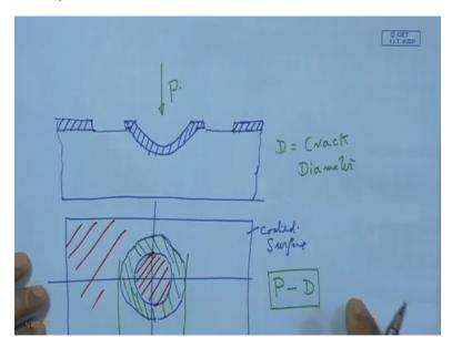
And in this case what is going to happen in case of poor adhesion, what we can find a portion which will be deformed so that means this is going to be a portion which is deformed like this. However, this will be the coating and here one can find out that means a crack formation that means there will be at this point the substrate will be exposed and low coating will remain so this will break and this will be separated from the substrate.
