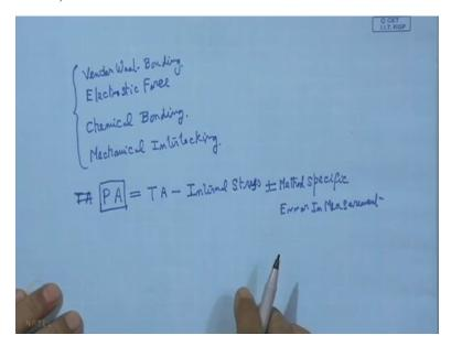
Now what we see that here actually we have various types of bonding, now one is Vendor Waal Bonding that is the physical adhesion, then we have electrostatic, electrostatic forces that also can bring them to together, then we have further to this Chemical attachment that means this chemical bonding.
