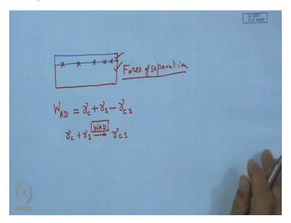
Now comes, Experimental Assessment of Adhesion, now here we have some interest in determining the value of this adhesion, either in terms of force or in terms of energy, that means if we consider this as the coating and the substrate here we have certain length and we can have the width normal to this paper, then definitely this adhesion that perhaps one can measure that this is a surface, length into the back engagement or the width.
