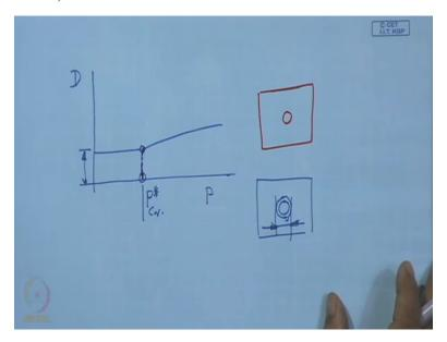
So this is about indentation test, now this Principles of Indentation Test that we have discussed and how we can use this PD characteristics and here one point we can also see, one point we can also mention that PD. So definitely as we get this curve, there may a point from where we get a crack diameter, so actually what happens below this we do not have any crack diameter so it is only indentation and from this point, so that means here the load is increasing.
