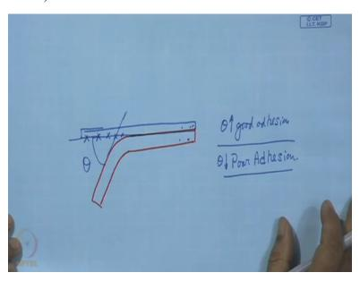
That means we can draw another figure to show that separation of the coating quickly we can show this, say this is the substrate and here it has undergone little bit of bending and however the coating does not remain with this one and it is something sort of thing which looks like this. That means from this part the coating gets separated, so this area the coating gets separated from this substrate surface.
