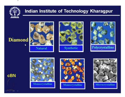
Here we see various types of diamond and cBN this is one of the natural variety which is mine one, mine diamond, this is synthetic man-made which is a single crystal type having a blocky shape very strong and tough these are used for difficult grinding task. Here we have also polycrystalline diamonds which are used for grinding delicate material just like Tungsten Carbide grinding where the work material is very sensitive to heat and force associated with grinding.
