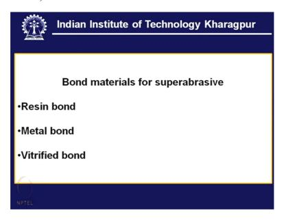
Now comes the bond for super abrasive material as we know that if it has to act like a cutting tool then this diamond or cBN these are the cutting tool. However the resin bond or the metal bond or even vitreous bond they are actually the tool holder. So very important issue here is that, this material during grinding should have adequate strength it should not crumble or crushed.
