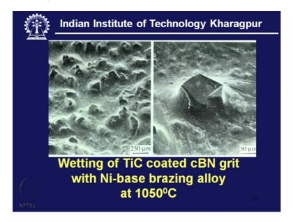
So this even this voids Micro voids which are well covered by this CVD, so this part could not be polished remain unaffected. So what we can see here? That the whole periphery is covered with this coating of Titanium Carbide and this Titanium Carbide really helps in improving the wettability.
