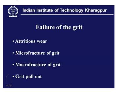
So here we see attritious wear, microfracture, microfracture of the grit these are all on the grit but this is exactly grit pullout that means as a whole the grit is removed from the bond's leaving just a socket or a pocket or it looks like a whole. So this has to be prevented at any cost.
