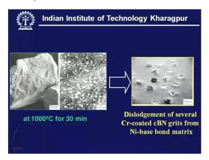
But here we can see that this CVD coating of Chromium can be also attempted on cBN and diamond. However what has been seen? That in this case this Chromium coating the result was not successful in that this coating was not appear like a continuous one, we have some island of this coating which appears to be a non-wettable.
