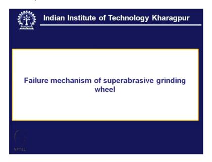
Now what is mean by failure mechanism of super abrasive grinding wheel? It has been well understood that in super abrasive machining or grinding the grit is a high-performance material. So this material has a very long service life it is in contrast to conventional abrasive. So what is very important in this case? That this grit material must be held with the strongest possible grip on the bond material and this grit should not have any premature dislodgement during the course of grinding.
