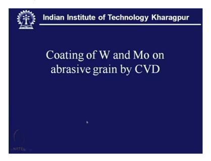
Coating of Tungsten and Molybdenum on abrasive grain on by CVD can be also applied and here of course one thing should be taken into consideration that the reactivity of this Tungsten and Molybdenum towards the cBN or diamond because unless this reactivity exists or a compound is formed then this coating process cannot be facilitated by this CVD operation.
