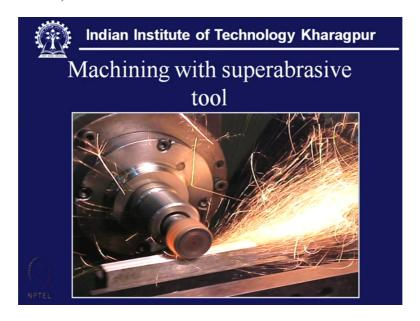
So this is one example of super abrasive machining engaging a super abrasive tool and this is just a steel core on which one of super abrasive grits are anchored or bonded and that works at a very high speed generating huge amount of spark but at the same time removing large volume of material which is comparable with that of machining but at the same time its surface quality which it is going to produce that is as good as that of grinding.
