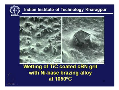
So in that case what we find? This material really has wettability. So this is getting wetted and this is clearly evident in this picture. So this is actually pulled by this coated surface that means this TiC coating virtually pulling this alloy thereby decreasing the interfacial surface tension.
