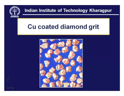
Here what we see? On diamond grit which are used for making one resin bonded abrasive wheel which is exclusively used for grinding of Tungsten Carbide which are used on the cutting tool, so it is one of the very delicate and sensitive operation that means the force or the temperature during grinding should not be allowed to rise I mean above a threshold value which may otherwise cause damage to the work piece.
