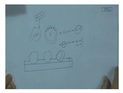
As we have mentioned that when we put this CBN grain on a substrate and here we have this liquid, this metal Nickel Chromium base alloy which was melted and after melting when it is unquoted it didn't wet the surface. So what actually happened?
