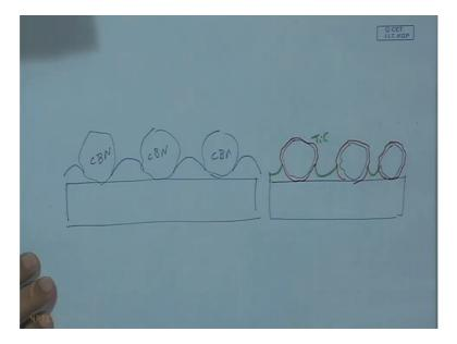
That after this melting, if these are the cBN grain after melting, so this is a substrate on which this grits are resting. So after melting we have a nonwetting profile of this Nickel Chromium alloy. So that means it did not wet cBN, cBN means unquoted cBN but when it is coated with this TiC. So now we have a TiC, these are the grains of cBN and here we have a coating of
