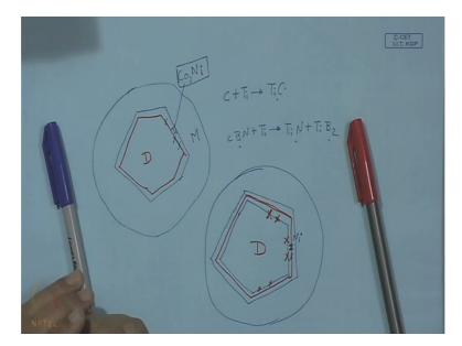
We can also have Titanium coated diamond grit. So in this case what we see? A diamond grit, of course these are the strongest grit, what we have seen? This is a blocky very strong and these are meant for many challenging grinding task using diamond. So here this is diamond, so outside surface is coated with Titanium, a coating of Titanium and just add is embedded in a metal metrics and this metal metrics ordinarily cannot have a chemical attachment as is the case what we have seen with cBN?
