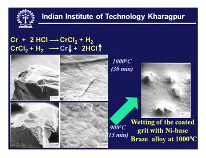
However when this was put on diamond the result was totally different and here even at 900 we could get a continuous coating which is in contrast with what we can see here and this one with 1000 they could have a crack because of the difference differential thermal expansion. So if it is handled with little delicacy then we can have a good coating of Chromium over this diamond surface then these grains are extremely wettable, very good wetting can be achieved
