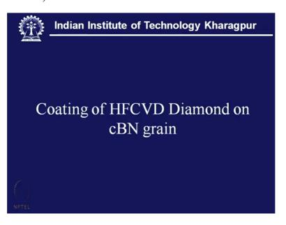
Coating of diamond and cBN grain can be also given in this case, what is going to be achieved? The diamond has good wettability towards many metals where cBN has shown its inertness. So a coating of diamond and cBN can be a good way of enhancing the wettability of cBN surface.
