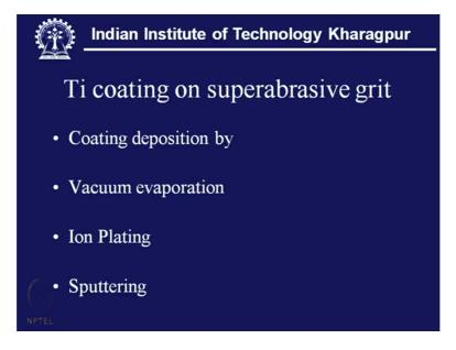
Now comes Titanium coating on super abrasive grit. So this Titanium coating is given by vacuum evaporation, ion plating or by sputtering. So these are all PVD processes, for Titanium CVD within a range of 1000-1100 is just not possible because of the chemical stability of Titanium Tetrachloride which doesn't allow one to reduce Titanium and here these processes are well matched with this grain coating.
