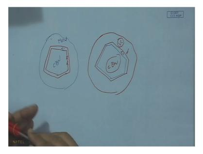
So it will be something like this, so this is the cBN grain and on that we have a Titanium coating. So this is one interface and it will be embedded in a metal metrics and this metal metrics normally is inert towards these highly chemically stable cBN. So inside you have cBN this is Titanium coating and here you have the metal metrics. So Titanium is making a
