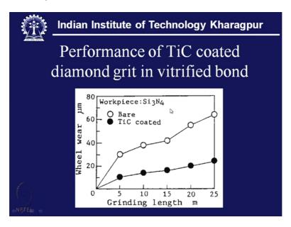
So here we can see immediate benefit that this one with this TiC coating and this is without TiC coating and this diamond was used for grinding of silicon Nitride, a material like silicon Nitride and what is very interesting observation? That just by virtue of this TiC coating the
