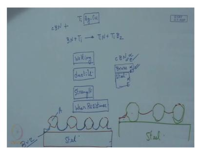
Suppose we have this grit material and this is the bond material, the steel substrate. So the braze alloy should have a balanced wetting towards the steel and also towards the grit. If there is not this balance then the interfacial tension, if there is too much difference in interfacial tension.
