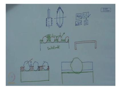
The idea is that in this case what we need? We just need a pre-form. A pre-form it can be any shape, so it can be machine with by precision machining and over that this grit can be anchored by this electroplating technique. So only the pre-form is necessary and we can do away with this moulding or the requirement of the moulding. So that is one of the greatest advantages of this technology.
