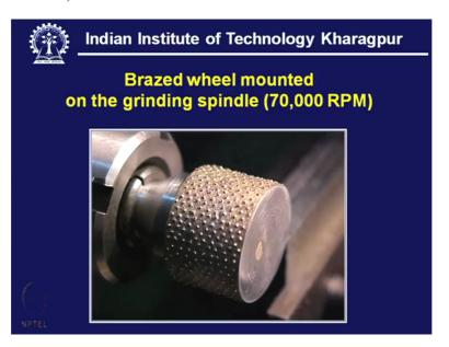
Now this is the outcome of this brazing that where the grits are implanted or bonded to the surface and it is actually the coating that means it is a coverage of the grit on this wheel surface in a monolayer formation and is written be located at a fixed distance thereby we can also maintain the gap between the grits, this is desirable from the requirement of grinding.
