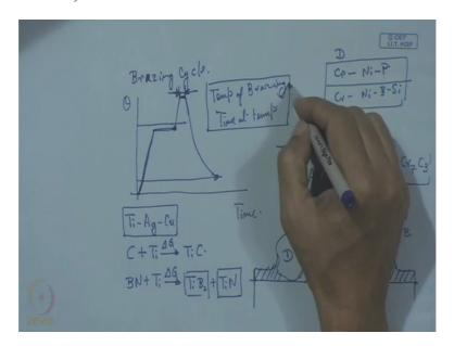
This one we get back to the slide that means this thickness of this reaction layer that can be properly controlled. So in summary what we can say? That this thickness of the reaction layer should be controlled by this brazing temperature number 1 and number 2 by the amount of this reactive element and the presence of one of the ternary element which can control in a very favourable manner that the of this reactive element.
