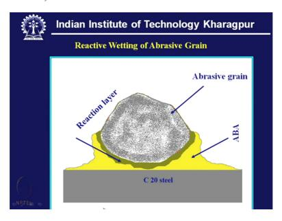
So what is important in this case, very important issue? That as we have mentioned that this is reactive wetting it's no more non-reactive wetting. So here we must have a reaction layer and that has been shown by this schematic figure that say this is one abrasive grain may be diamond or cBN and this is a low carbon steel substrate and this green is held over this steel substrate.
