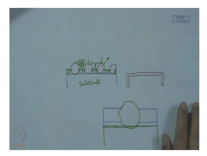
And for that we have a new concept and that is exactly what we call? Monolayer abrasive tool and it is going to offer a solution to this aforesaid problem. So monolayer abrasive tool basically what we see here? That as we have mentioned at the very beginning of this discussion that means on a substrate it can be say for example this is metal substrate and over that we have the grits.
