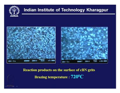
So here we see that this is the very strong reaction showing this needle like thing titanium di boride and it's a very strong reaction with a alloy having almost 10 percent titanium and temperature 920 degree whereas when it is at 720 we have this reaction but it is a mild reaction thickness is also very low and it is good enough to have a very good wetting but at
