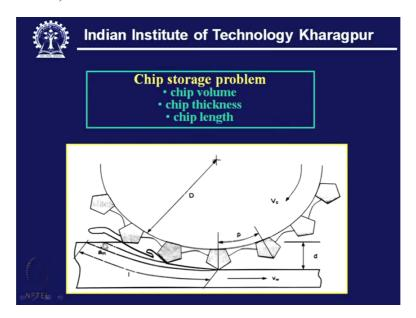
Now wheel depth of cut is quite small compared to the diameter of the wheel and in that practical purpose, what we find? The volume of the material removed by each grit that means this grit starts its actions from this point and that is the kind of this grinding action it repeats itself, however there will be series of this grit arranged over the entire periphery and each has its own cutting action and the volume of the chip that will be given by am into L, this is one thing.
