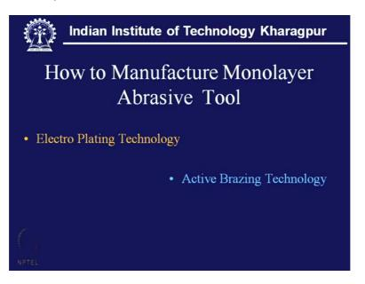
Now comes the question which has been raised, how to manufacture monolayer abrasive tool? There are actually 2 technology for making such thing, one we called Electroplating technology another is Active Brazing technology. So these are the 2 available processes
