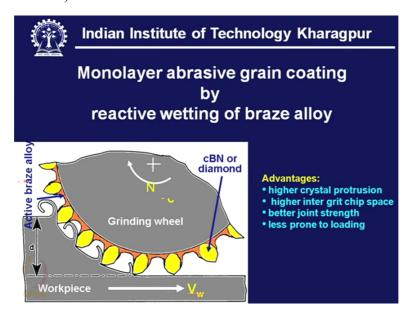
Now this limitation of galvanically monolayer abrasive wheel which has been just now highlighted because it is at least 70 percent coverage that can be reduced to 20 to 30 percent coverage by this brazing technique, so what we're doing here? We are not changing neither this material this core, core area of the wheel which is steel special steel according to the need of grinding also the same grit material it remains as it is.
