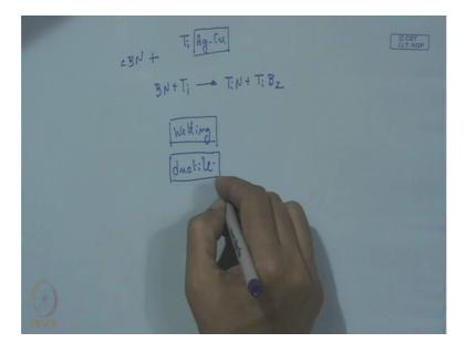
Now requirement of the bonding alloy, now what are the requirement of the bonding alloy? Obviously it should be wetting number 1; the necessary condition that is the wetting, the material must be also ductile. This ductility is also one important term in that, unless the material is ductile there will be tremendous amount of thermal stress. At this brazement it is because of the simple reason that ceramic though it is very small it is cBN and on that other side we have steel.
