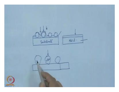
But in this case with one layer configuration re-sharpening of the grit is just not that easy and this single layer configuration that will keep on providing the grinding result which is more or less uniform throughout the grinding span.
