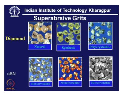
Here we see the super abrasive grit, look this is a natural diamond and it is mine diamond. So from the mine the non-gem quality of diamond that is separated and then through this use of the crushing technology they are properly screened and sized but each grit has a multifaceted appearance. Basically it's a fractured surface but then there may be some post crushing, polishing process which can little smoothen the surface.
