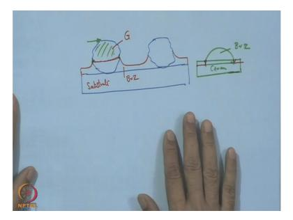
So this is just not free of any problem and then most importantly the thermal residual stress and this is very important issue but as to care for, say it can be illustrate by this simple sketch, this is one grit this is the second one and which are being supported by the substrate material and here we have the braze alloy and these base alloys by waiting effective waiting it will give this shape.
