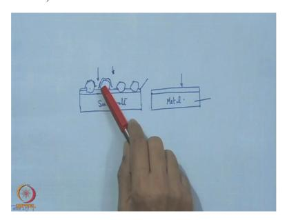
There can be another way of doing the thing that there are certain process which are practiced in industry that means these crystals are coated with a non-conducting coating like a plastic coating and then the so-called conducting grit may lose its conductivity and without any difficulty that can be used for anchoring on this surface. However the surface is smooth as we see it is perfectly grown crystal.
