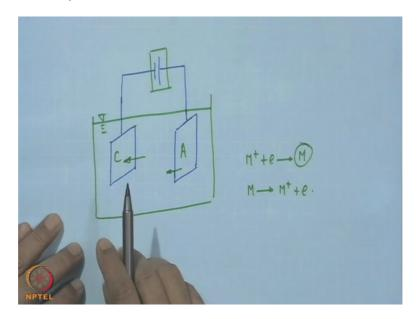
Now the principle of electro plating, we can have a quick look to this electroplating. So what is going to happen? Here actually we have one plate which is going to serve as the cathode and we can have another plate which is going to serve as anode, so they are properly polarised and these are actually put inside an electroplating bath. So this is cathode and this is anode.
