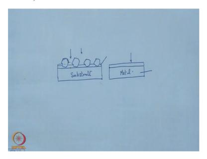
If we have just multifaceted surface then this will help in Anchorage of the grit in the bond. So this is natural diamond, so one requirement is that there should not be any electrical conductivity number 1 and number 2 if we have a rough surface that adds always to our advantage enhancing than Anchorage of this Electro deposited metal on the surface of the abrasive.
