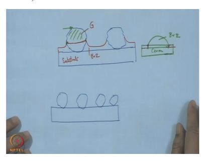
Now as we have already seen that this is going to be one layer configuration, so it is going to be one layer configuration and it is not very similar or identical to conventional wheel where you have more or less of composite mass. So when it is a moulding process or moulding practice, what we take normally it is a mixture uniformly mixed this combination of the Bonn material and the grit material that forms a composite mass.
