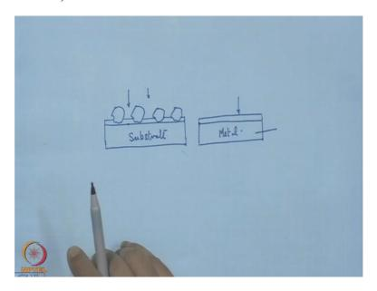
Now requirement of the abrasive material, now this material one point we should consider that this material is going to be in the metal bond and this metal bond is an Electro deposited bond that means this material of the substrate that should be electrically conducting the substrate material.
