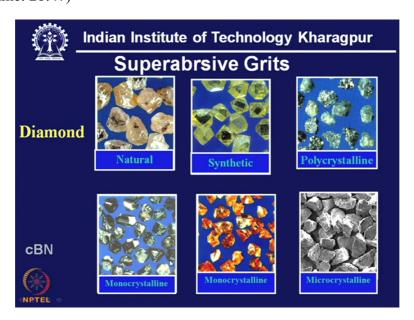
Now when we look at this cubic boron nitride, here also we have 2 type of crystals Monocrystalline and Microcrystalline and Monocrystalline this black variety is very strong, here boron percentage is retail more than that of nitrogen and here it is amber colour when
