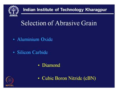
So it is a well dispersed mass of the structure but in this case it is a single layer formation. Now when it is a composite mass, it is not the abrasive wear resistance there is not a big issue because of the simple reason Aluminium Oxide, it is known Aluminium Oxide is inferior to Cubic Boron Nitride or Silicon nitride, Silicon Carbide is also inferior to diamond, so far as grinding ratio is concerned or wear resistance.
