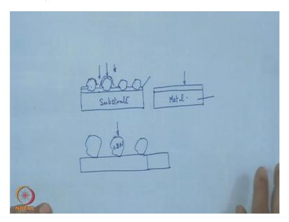
So on the surface if we place this cBN particle, cBN and if it has excess boron then that could become a problematic in that surface boron which is excess surface boron which can also lead to electrical conductivity and in that case also the position of this galvanic metal from this electrolyte that is that cannot be just ruled out. So what is to be done and what is done also in the industrial scale?
