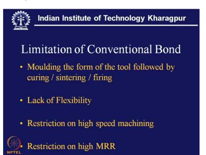
However the conventional bond their limitations are soon realized and these are few which are highlighted here, to make this wheel we need one mould and this moulding gives the shape of the form which should follow this what we call curing or sintering or even firing depending upon whether the bond is resinoid metal or vitreous.
