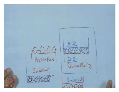
Now reverse plating, this reverse plating is important in that it can it facilitates making or Manufacturing of precision abrasive tool. So here we have to have a dummy substrate the basic principle like this in normal electroplating the grits are place like that and if this crystal heights are not same then these pick points are not on the same height. So they cannot have uniform cutting action.
