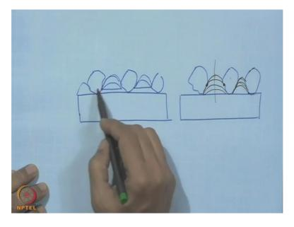
So here actually these are anchored this is just not a deposition what we understand by classical means but it is just the placement of crystal and then it is actually the deposition of the galvanic material and it is holding by proper Anchorage. Now here what we can do? Normally what we see that nickel is used as the plating material. So here we have the grit and this is the platable material, the nickel is known for its platability.
