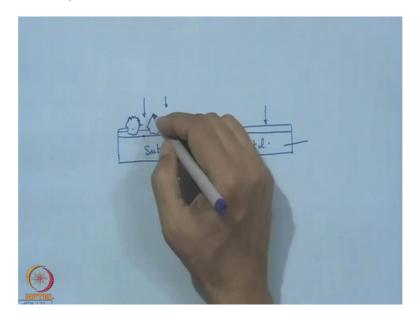
And if in unfortunate eventuality some of this catalyser like a solvent remain on the surface and that is not removed and it is overlooked then that can become a path or the source of conductivity and if this conducting path is created when this is placed on the substrate then there is every risk that this metal which is not supposed to sit on this surface that will deposit over and it may in certain extreme situation it can cover wholly or partly the grit and there will be heavy metal deposit.
