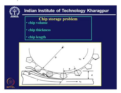
Then we also find restriction on high material removal rate and this can be understandable if we look into this figure. Now here we have the grits which are arranged over a periphery and this is the space available ahead of each grit or the cutting tool and this space must be adequate in order that this volume of chip which is shown here, this volume of chip can be well accommodated and once this chip pocket lips this workspace surface, then it will be thrown out by centrifugal action.
