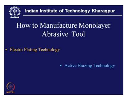
Now there are 2 ways of doing the thing either Electro plating technology or active brazing technology and by adopting one of these either plating or brazing, one can realize this abrasive tool with his monolayer consideration. Now each has its own merits and weakness.
