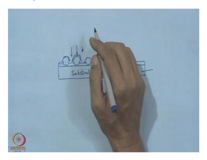
So we find that though synthetic crystals have many advantages but this user selection cannot be obvious and here utmost care has to be taken, so that this can be well anchored in this bond and at the same time there is no material deposit on this crystals surface because of some inherent conductivity and it is due to the presence of this catalytic agent which are used during the synthesis of diamond.
