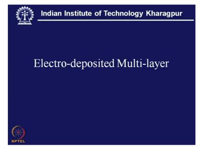
Now this is electrodeposited multilayer that also we have mentioned, that a chromium coating over a nickel coating that can be used for this purpose with a view to enhancing the wear resistance or some tribological property.
