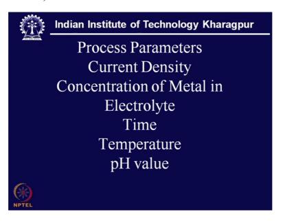
Now one thing we have to also look, that what are the process parameters of this electro plating technology. Now here one is definitely the current density, current density means on the electrode surface this current is collecting and the area over which so much of amperage is supplied that gives the current density. So par you need the area, what is the current density?
