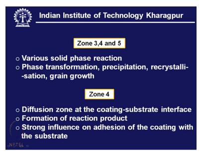
We have Zone 3, 4, 5 where various solid phase reaction may take place. And this can be phase transformation, precipitation, recrystallization and grain growth.
