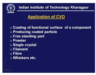
Also, instead of a (cover) coverage or having some dust, one single crystal can be also grown and it can be also used in various application. A filament, say for example, a tungsten filament can be also made by this process. It can be as an extension of the CVD, we can also use it for making fiber or whisker. (Refer Slide Time: 5:24)
