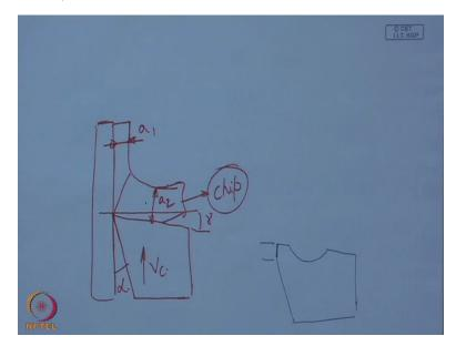
It means that originally the tool is like this, what I have already shown. So this is actually the rake angle, this is the clearance angle. And it is actually the chip which is flowing from this side. So here we see that rubbing action, one rubbing action between this finished surface and the side
