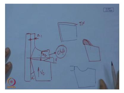
That means here we have the tool, the same tool and we put a coating of titanium nitride over this. And this coating of titanium nitride now protect it will protect the tool and wear resistance, it will take to a greater height. So this tool which was non-performing, now become a high performance carbide tool just because of a titanium nitride coating, maybe 4 to 5 micron thick.
