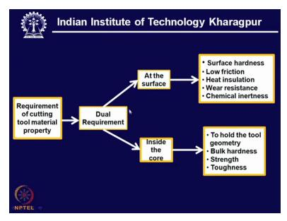
And what has been correctly identified in this case that we must have a dual property and this dual property means we have to have sharing of the responsibilities between the surface and the inside core area. And these are the responsibility, this is the responsibility of the surface to provide these properties, characteristics and that had been the task of the core area to hold these characteristics.
