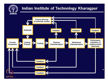
Now we see the overall activity in the domain of coating technology. We see, we start with the substrate. Substrate material once it is chosen, we have to precisely tailor the substrate surface so that it becomes a good receptor surface. That means the coating material should be received, well
