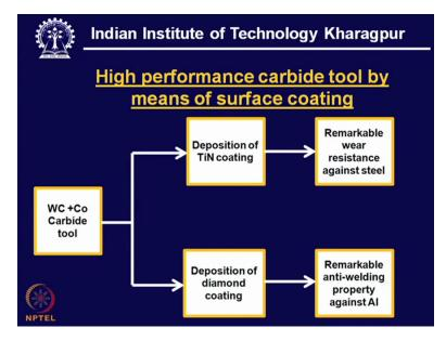
The solution is here. We have now from this ordinary tool, this limitation is overcome. We have high performance carbide tool by just means of surface coating. So this is the carbide tool. We have a deposition of titanium nitride coating.
