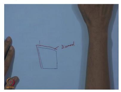
Similar is the case with this machining of aluminum. We can also see here that this is the same carbide tool which was used with lot of limitation, shortcomings but now those will disappear. Just we put a coating of diamond on the surface. So this is diamond coating and we can
