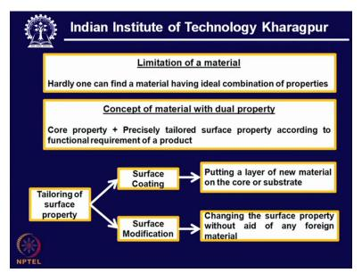
Now comes the very limitation of the tool material or any material. So what we see hardly one can find a material having ideal combination of properties, so that is why we have to go for this concept of material with dual property. It means exactly what I shown already.
