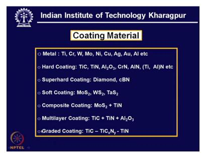
Coating material, these coating materials, it can be from metal family, it can be from hard coating. This metal family, these are used in any mechanically functional surface mostly for improving either the coefficient of friction or to increase brazability or wettability brazing. Then
