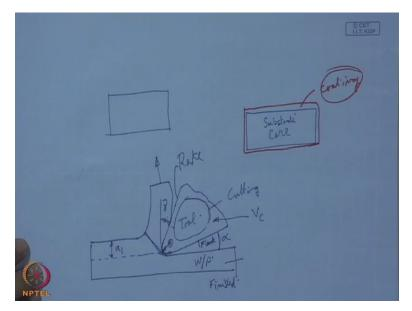
That means if we have, this is the core material as received and on that we can put a coating of another material and which has the required surface property. So this is actually the core or the substrate, we also call it substrate. And this is the coating, so this is actually the coating. So this coating material having those desired properties as we have mentioned in reference to the cutting tool it will offer.
