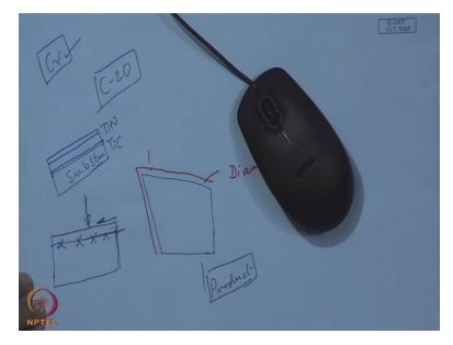
That means from the substrate we start with TiC and the top may be TiN, this top layer TiN. But we must, this is TiC, and we must gradually change the composition for various reasons. And in between we can put some (oxi), some carbonitride coating also. So these are the various coating materials which can be used to improve the surface property or to make the material high performing.
