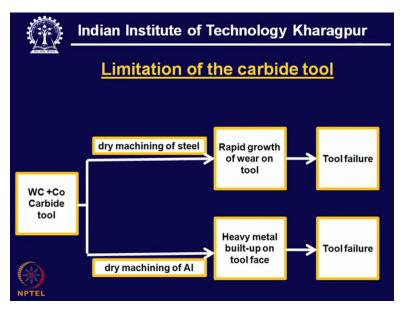
But what is important to look at? When we use such carbide tool to have some machining task, so this is actually the limitation of the carbide tool, one can immediately recognize. We like to have dry machining of steel and we can see rapid growth of wear on the tool which leads to tool failure.
