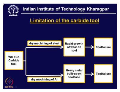
But these two tools just cannot work under this condition. If we go for high speed machining or dry machining of aluminum, we can say that this tool are going to fail and how to get rid of this problem or offer a solution?
