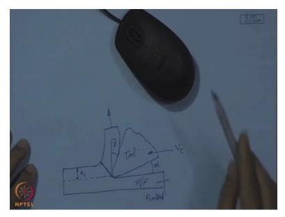
This is the cutting tool and here this is going to be the workpiece. And this is actually the cutting action, so more or less this is the cutting action. This is the tool. This is the workpiece. It is of course, this is the finished product, finished. And this is the original material and here what we
