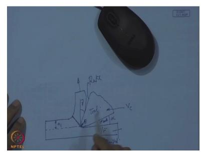
Now let us emphasize on this role of the cutting tool. So it must have both micro geometry and macro geometry. Micro geometry we mean that this edge where the flank of the tool, this is called the flank of the tool and that is called the rake surface, these are meeting. So they are actually, there is a continuity by providing a edge rounding radius. So this is going to be an edge rounding radius. So how to choose this clearance angle, rake angle and edge rounding radius?
