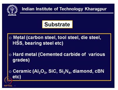
Substrate, substrate can be metal which are used mostly in functionally, mechanically functional material: carbon steel, die steel, HSS, bearing steel. In the hard metal family, we have lot of substrate. In the ceramic family, we are also having, few things we have mentioned here as for illustration.
