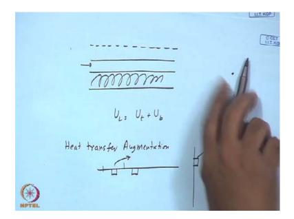
You have the glass cover and the duct through which the flows and of course, you have insulation. So, here is U L equal to U t plus U b. So, there are no issues. So, you have that a F dash efficiency factor and the radioactive heat transfer coefficient. And this is to have a heat transfer augmentation particularly for air collectors people provide sort of.
