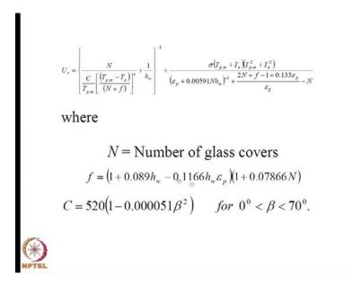
This has been correlated by claim in terms of the number of glass covers the wind heat transform coefficient emissivity of the plan of the plate emissivity of the glass mean plate temperature ambient temperature and of course, Stephen Boltsman's concept and where this f and c are again in terms of other quantities like beta the slope.
