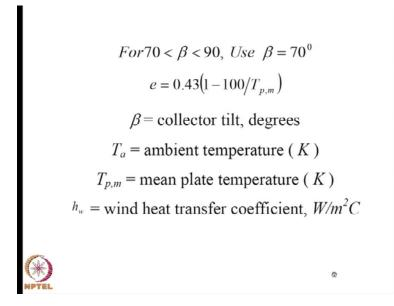
And everything is explained over here. So, this can be readily used and then you can calculate U t U L as U t plus U b the black loss coefficient which is nothing, but the resistance inverse of the conduction or the insulation kept at the bottom of the absorber plate.
