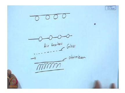
And very first configuration we studied was with the tubes below the absorber. And this one is above the absorber.
