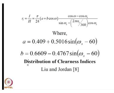
So, this is in addition to the same term of I d by H d you have got in terms of pi by 24 times a plus b cos omega times cos omega minus cos omega s up on sin omega s minus 2 phi omega s by 360 cos omega s. And you should remember omega s is n degrees.
