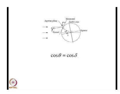
And cos theta is given by simply cos delta the figure is shown over here and you can see that depending upon the equator and the plane of rotation which differ by an angle delta my cos theta will be equal to cos delta. Which is pretty good compared to perfect tracking where you have got cos theta is equal to one.
