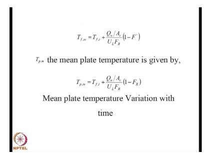
Now you can express fluid mean temperature T f m as T f i plus the Q u by A c it is only a rewriting of it not that you can really calculate by this equation you cannot do that unless you know Q u. and the plate temperature is T f i plus same thing Q u by A c by U L into F R times 1 minus F R .So, subsequently we have analyzed for a number of other configurations not just final tube, but different arrangements for the liquid based as well as the air based collectors.
