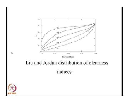
So, they have given cumulative frequency or fractional time verses K T daily or hourly or I will write small K T. This is for K T bar equal to 0.3 this may be for K T bar equal to 0.7 this may be approximately one and this is 0. So, what basically it means is if you take a month for example, there are 31 days or 30 days. So, you have daily clearness indexes.
