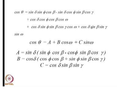
So, that theta in general a function of the latitude slope and of course, the time omega and the azimuthal angle gamma is a long relation which can be put in a shorter form as cosine theta equal to A plus B cos omega plus C sin omega where A is this expression and B is another expression and C is cos delta sine beta sin gamma.
