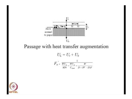
Corrugation or the paths in between. So, this will break the sort of boundary layer or mix the hot and cold fluids from the bottom and the top between the duct thereby improving the heat transfer between the fluid and the absorber plate. So, this is analyzing terms of the spacing h 1 and h 2 are the heat transfer coefficient and the expressions are over here. (Refer Slide Time: 41:34)
