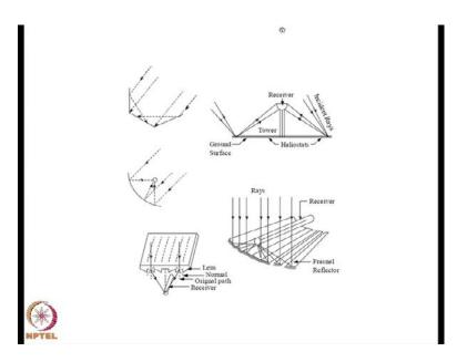
Concentration methods which you may find it here is simple rather they are something like two boosters and then you may have the central receiver concept or a parabola idol dish at the focal point being the receiver and the Fresnel lens or a Fresnel reflector. So, the necessary condition for a concentrating collector is they need to be tracked.
