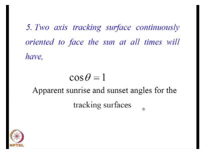
Because, delta maximum is only 23 degrees and which will be almost 0.95 or. So, consequently cos theta being about 0.95 or higher compared to cos theta being to equal to 1 that is not much of a loss in having its only single axis tracking compared to perfect to axis tracking. So, in all these cases we need to calculate the what I shall say the apparent sun rise and sun set hour angles for each mode
