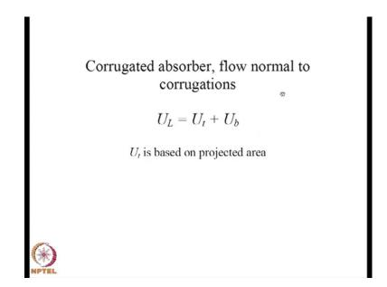
So, here also its not directly coming in contact with a heat losing surface. So, U L equal to U t plus U b. So, this is a insight the tube which we have done then f dash the collector efficiency factor is given on here.
