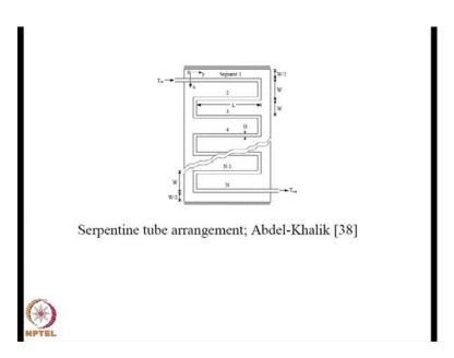
Given over here serpentine tube arrangement the advantages it had got the fin efficiency plus also at the of the pressure drop though the entire fluid will be going through the pipe. There by your heat transfer characteristics may be better though there will be additional a pressure drop also this is done by Abdul Khalik. So, these relations we have given in detail in the class notes on the earlier lectures. (Refer Slide Time: 44:01)
