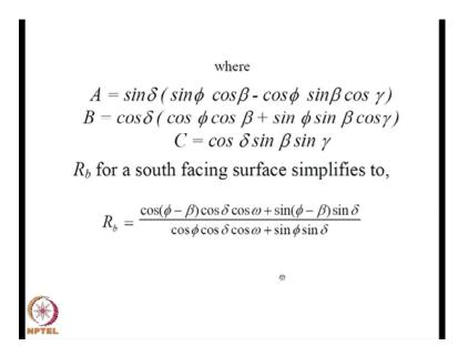
And then where A B C are given and R b for a south facing surface is simple like R b equal to cos phi minus beta cos delta cos omega plus sin phi minus beta sin delta by cos theta z which is cos phi cos delta cos omega plus sin phi sin delta. So, these relations are I am giving it again and again. So, that you should become familiar not be just afraid to
