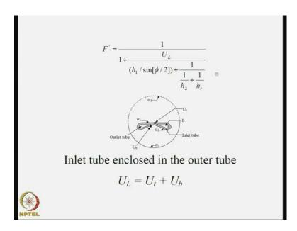
So, this is a insight the tube which we have done then f dash the collector efficiency factor is given on here.
