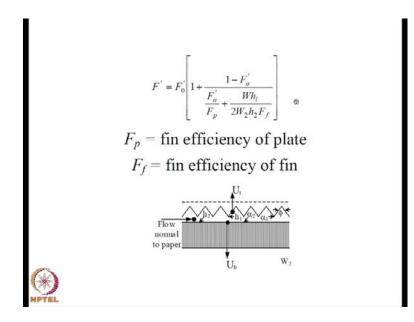
So, now, you can define the fin efficiency of the plate and fin efficiency of the fin because when I talk about these two this the fin efficiency of the plate and if you take this as a fin this is the fin efficiency of the fin. Now, people try to improve the heat transfer characteristics particularly for the air arrangement by having the flow through a corrugated sheet.
