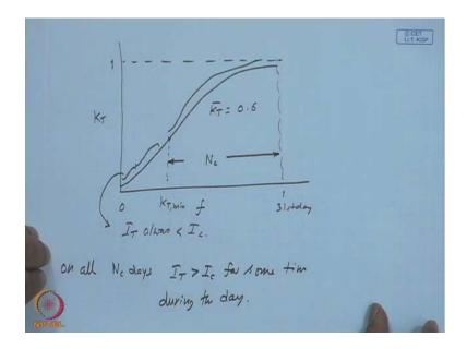
In other words, if I have got K T1 to K T 30 for 30 days whose distribution according to Lui and Gord Ankers cumulative frequency versus K T for a given K T bar say 0.6. This approximately 1 and this is my K T minimum. So, this much fractional time, I T always is less than I C. In these fractional times or the number of days, this one is accumulated to frequency or it can be considered as 0th day and 31st day. So, in these N c days on all I T is greater than I c for sometime during the day.
