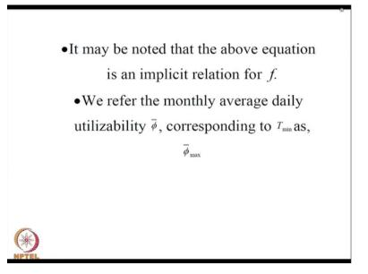
So, if you want this, require iterative calculation, a good guess first is slightly less than phi bar max y. This is calculable quantity. So, you know phi bar max. Let us say it is 0.58 and then I may guess f 1 as 0.5 phi. Then you can set up a Newton Grayson scheme or whatever, and you can easily interpolate or rather iterate in this relation to find actual solar load fraction met.
