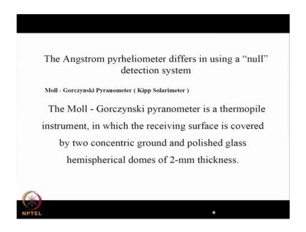
There are other types of pyranometers. This is moll gorczynski pyranometer or kippsolarimeter. This is a thermopile instrument, which has got of course, 2 concentric ground and polished glass hemispherical domes of 2 millimeters thickness.
