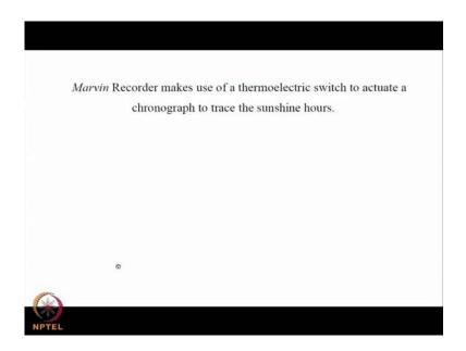
Marvin recorder makes use of a thermoelectric switch to actuate a chronograph to trace the sunshine hours.
