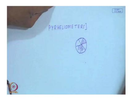
The circular disc, which is brightly polished instead of being surrounded by another black one, it is alternately painted black and white or polished. So, the temperature difference between these types of sectors is measured. So, this also basically is the temperature difference between the brightly polished and black painted surface.
