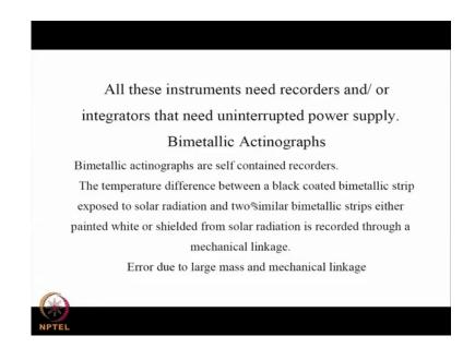
There is another instrument called bimetallic actinograph. These are self contained recorders because essentially they depend upon the displacement of length of a black coated bimetallic strip exposed to solar radiation. The other bimetallic strip is painted
