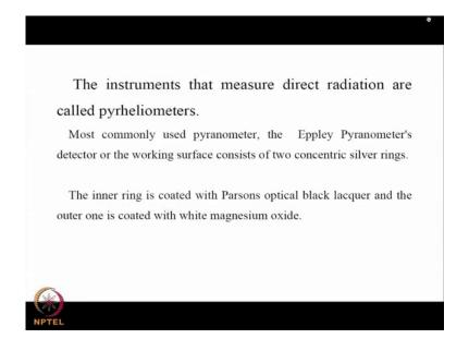
It basically shadows the sensor from the direct radiation making it record only the diffused component of radiation. You can understand the difficulty associated in measuring direct radiation is that the instrument has to be directed towards the sun. Such instruments are called pyrheliometers.
