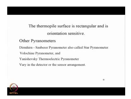
The thermopile surface is rectangular. Hence, it will be orientation sensitive. Normally, this is called a second category of instrument compared to eppley pyranometer. Of
