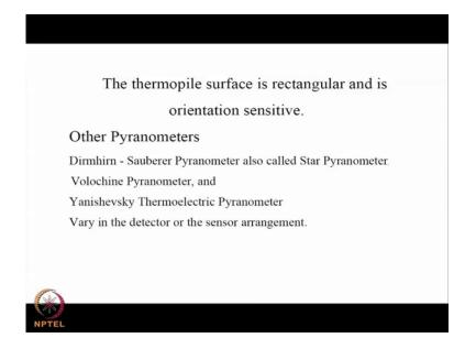
One is the Dirmhirn Sauberer pyranometer also called the star pyranometer or a Volochine pyranometer and yanishevsky thermoelectric pyranometer. They essentially vary in the detector or the sensor arrangement. The sensor could be rectangular sensor. It could be circular and the detector could be thermal detector or photon detector and sometimes circular.
