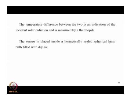
This produces a temperature difference between the black coated being at a higher temperature and the brightly polished material being at a lower temperature. The temperature difference is measured by a thermopile, which is connected to a measuring device like a microvolt meter or a milli volt meter.
