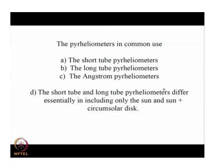
The pyrheliometer is basically of three types, the short tube pyrheliometer, the long tube pyrheliometer and the angstrom pyrheliometer.
