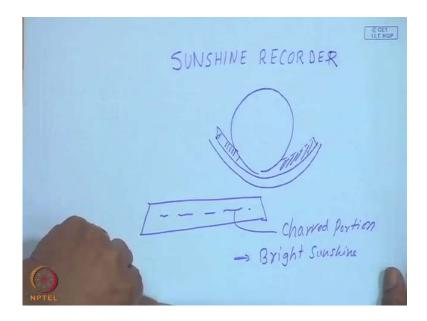
It also has a reliability though may not be as expensive. It may not be as accurate as the pyranometers or pyrheliometers. This is simply a spherical length arranged in a bowl and
