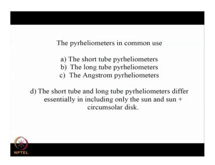
They are the short tube pyrheliometer, the long tube pyrheliometer and the angstrom pyrheliometer. The short tube and long tube pyrheliometers essentially differ in measuring either the direct radiation coming only from the sun or from the circum solar disc round the sun.
