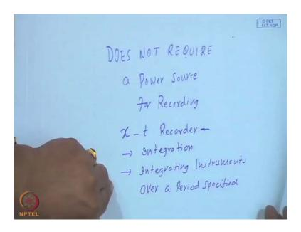
This does not require require a power source for recording. For example, if you have a pyrheliometer or pyranometer, the solar radiation needs to be continuously recorded. In the olden days, it used to be some sort of x t recorder. If one wants to get a value for 1 hour or 1 day, it goes through a painful integration process quite often mechanically or using a plan meter.
