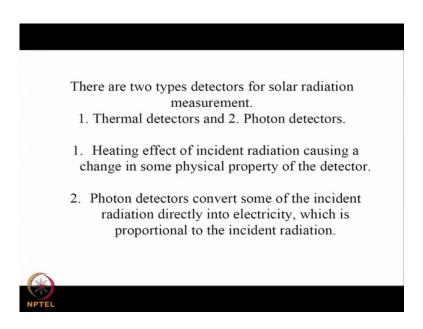
In terms of detector, perhaps more easily and more widely measured meteorological or other variables, basically the solar radiation measuring instruments make use of 2 types of detectors for solar radiation measurement. One type is the thermal detectors.
