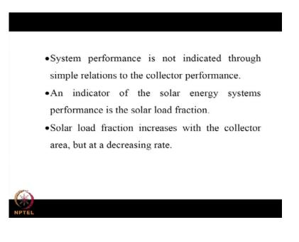
So, that is we are getting is a load fraction and this solar load fraction increases with the collector, but at a decreasing rate.
