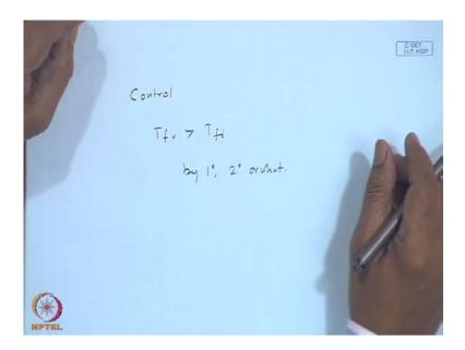
If you consider the control, so that T fo is greater than T fi outlet temperature from the collector is higher than the inlet temperature. How much? It is by 1 degree, 2 degrees or so. If you put the thermostat in the control, actually you will find that it is turning off or turning on the pump with 5 minutes or 5 degrees are band width compared to another control which may have a band width of only 1 degree, ok.
