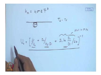
And this is of course we can express the radiate to be trans coefficient in terms of 4 sigma epsilon some T bar to the power 4, whereas we have already defined it is a average temperature of the receiver T R and the surrounding ambient temperatures T a in terms of the fourth powers.
