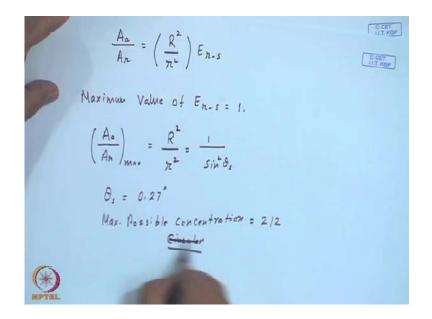
So, that gives us A a by A r equal to R square by r square times E r s. Now maximum value we were estimating the theoretical maximum, so I can assume this of E r s equal to 1. So A a by A r max equal to R square by R square equal to 1 by sin squared theta s. So, if theta s equal to 0.27 degrees maximum possible concentration will be 2 1 2, that you put in the value of theta s you will get 212. This is for a circular concentrator.
