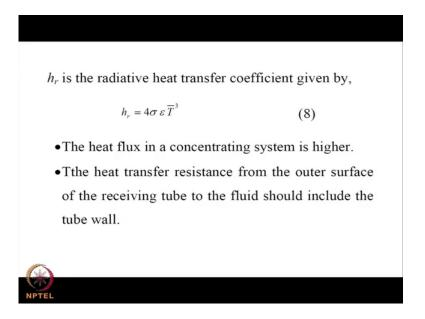
The heat flux in a concentrating system is higher, or the heat transfer resistance from the outer surface of the receiving tube to the fluid should include the tube wall. If you recall in our flat plate analysis that T b minus T f has been expressed only in terms of heat
