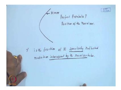
And depending upon your manufacturing technique, the mirror over here may not be perfect parabola. So, consequently, there will be some angulations, because it is a large surface. So, all the reflected radiations may not be striking the receiver. Then position of the receiver itself, there may be imperfection but most of it is due to the tracking not being perfect, and this manufacturing large or reflecting surface may not be following exactly the parabola that optics requires.
