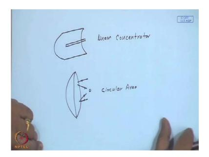
So, if you have a parabolic system, like we have drawn now, the attempt is to focus on to a line. So, this is a sort of linear concentrator. The other way around is if you have a parabolaidal, this will try to focus on to a circular area. So, technically this can be a point, this can be a line, or is it possible? So, which we shall show the possible maximum.
