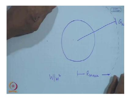
If this is the sun surrounded by a sphere, which is at mean distance between the earth and the sun, and you take any ray and you place a surface normal to the sun's ray. The amount of radiation received by the surface of unit area, located at one sun to earth mean distance is the solar constant, which is G sc that is, in watts per meter square. So, if we multiply by the total surface area at that radius, will be the total limited solar radiation by the sun.
