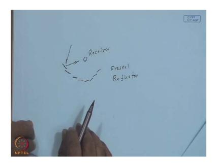
Similarly, you can arrange even the mirrors like this and on to a central tower so, so you have sun's rays reflected on to this. Now, the advantage of this type of smaller reflectors, as we have shown in the case of heliostats or this fresnel reflector. Each one of them can be tilted depending upon the sun's position so, this is a receiver, not to get confused with the sun. So, you need some sort of a orientation or tracking of smaller pieces of reflectors than one large piece.
