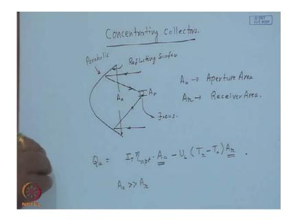
So, we go on to the next topic of concentrating collectors so, we explode improving the efficiency or the operating temperature for the flat plate collectors through 1 or 2 or more glass covers, platter insulation and even evacuation though, it may or not be practicable or to have a completely evacuated flat plate collector. So, the next idea is to have, what we call concentration and the very early type of concentration, you can see it in the form of mirror boosters.
