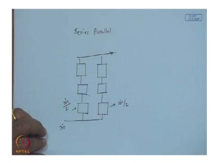
So, one can think of a combination of these things, series, we have considered parallel, we have considered and series parallel. So, 3 collectors over here, they are in series and they are in parallel with another 3 collectors that means, my original six collectors have been connected like this. So that, if this is my m dot, this will have m dot by 2, this will be having m dot by 2.
