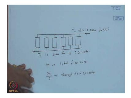
One way is, I will take it for the time being just 6 collectors, so let us say, there is a large header connected to this, connected to this, connected to this and all the 6. Then, again the delivered hot water will come out through these 6 collectors and I have some sort of a pressure balancing.
