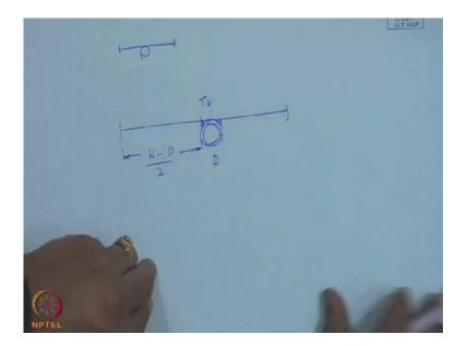
Then we have gone through the analysis, considering a repetitive element of a tube, and half a plate on either side, with the distance being W. Let me draw it bigger. There will be inside diameter D i, and outside diameter D. This is the repetitive element, and this distance is W minus D by 2, if the diameter is D, and this is at a temperature of T b, and this is bounded by soldering, or welding to be tube. We have subsequently considered an elemental volume.
