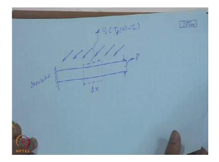
In the let us say the fin area, the mid plane choose the temperature is maximum, can be considered as insulated, with the element being shown, of elemental length delta x. In general this is receiving the solar radiation, and it will be losing also heat, by a loss coefficient, times T p, function of x minus T a, this p is unnecessary, it is a function of s and the thickness of this, is delta; not to be confused with the declination, they do not appear at any time, the same time.
