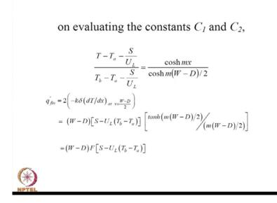
And if you apply the boundary conditions; that d T d x is equal to 0 or d psi d x is equal to 0, or psi equal to T b minus T a minus S by U L, you will obtain the temperature solution as T minus T a minus S by U L by T at the base, minus T a minus s upon U L as cosine hyperbolic m into x by cosine hyperbolic m into W minus D upon 2. Now we got the temperature distribution in the x direction at a fixed y.
