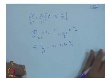
This quantity, if you take the limit and x plus k delta d T d x at x plus delta x. You will get an equation, d squared t by d x squared equal to u l upon k delta times T minus T a minus s upon U L. You can check all of them have the same dimensions of temperature, and the two boundary conditions should be d T d x at x is equal to 0 0, and T at x is equal to W minus d by 2; that is at the base of the pipe, or the tube will be equal to T b. And of
