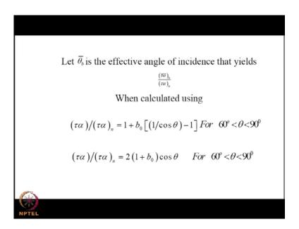
So, having got this tau alpha bar b by 2 alpha n, whether it is calculated using the beta or whether it is calculating r t and r d correlation, they have put back in the relation for 2 alpha bar n by tau alpha normal.
