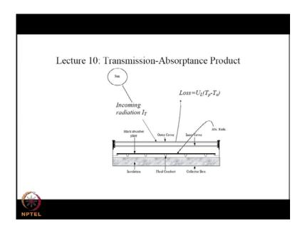
Particularly in order that we bring out the transmittance absorptance product, that would be required in calculating the performance of the solar collector.
