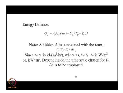
And will be absorbed and there will be several multiple reflections between the glass cover and the observer plate making that tau alpha within brackets, which I shall call the effective transmittance absorptance product, which is not exactly equal to simply the product of tau into alpha.
