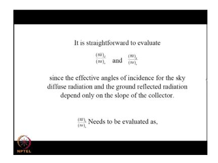
So, this I have already mentioned that alpha bar d and alpha bar g can be evaluated when once you know theta d and theta g which are simple functions of the slope of the collector and this needs to be a weighted average.
