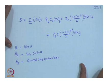
Now, this SR radiation S is given by incident radiation multiplied by effective transpative product. Now, we know that this I T compels of direct radiation and sky diffuse radiation plus ground defected radiation, we can say that the direct radiation strike the surface at the angle of incidence theta.
