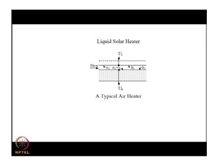
So, I have shown a typical air heater configuration also, where in you need a large flow area, because the volumetric flow way of air will be much larger for a given amount of energy gain compared to that of a liquid or water. Again this will be a duct and perpendicular to this the air flows and it is insulated. This is only to understand that the incoming radiation I T for which we have made elaborate calculations will be transmitted through the glass covers.
