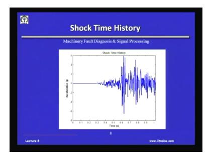
This is just to give you an another example we are talking about in vibration isolation yes this is a typical case of a shock which occurs in a machine and this is how it looks in the time domain and this values are actually -6 to 6. Well these are actually values measured from an earthquake and this is the ground and this is a very, very low level of; I mean this levels could be 25G okay.
