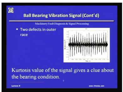
I will see the case when there are two defects. So, we made two defects this severity of the bearing increased defect increase and the values are very, very high .5, .4 and you see the nature of this so just by a time demand visualization of the feature of the of the signal we can say well something is good or bad in the bearing okay. But to be more correct we can always estimate the kurtosis or the RMS time kurtosis and then find out the such conditions of the bearing.
