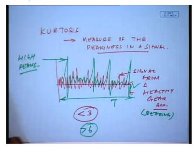
Kurtosis is actually is you can quantitatively say it is a measure of the peakiness in a signal. I will tell you how to calculate this either in Excel or in software known as MATLAB. So, for example if I have a real signal from a good gearbox it may look something like this okay. The red one is a signal from healthy gearbox okay.
