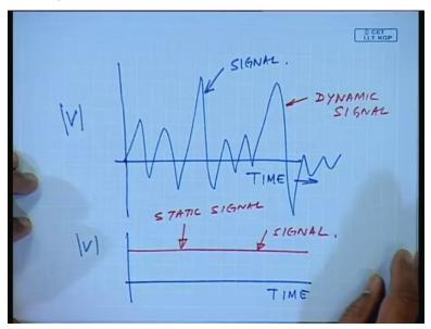
So, what do we see in an oscilloscope? So, in an oscilloscope we have our time base and then we have certain voltage which corresponds to the level of the signal and the signal could be of this nature varying with time so this is my signal. I have drawn the signal as varying with time but the signal could be at a constant level as a function of time.
