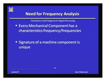
So, with this kind of on background you will see that you know well it is good that by time domain analysis we have some idea about the features of the machine. Sometimes you will see that we need to do a frequency analysis of the signal because of the fact that every mechanical component has a characteristic frequency, character frequency or frequencies is okay.
