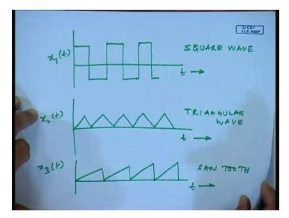
But there are signals which could be looking like this x1 t, so this is what is known as the square wave okay, signals which look like this, this is a triangular wave in fact there are commercially available signal generators where in you can electronically produce such signals either two calibrated equipment or to do check your equipment etcetera this can be done. And we will be using these waveforms in later on to understand the frequency domain analysis.
