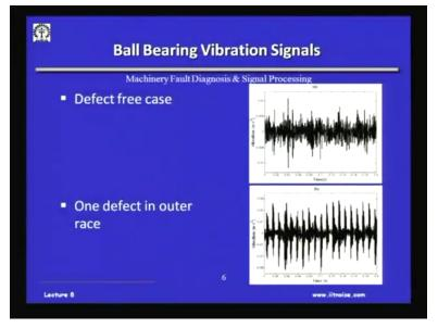
I will now show you some signals real world signals which occurs in the machine for example this is for the ball bearing signals okay and this is in time domain about 0.2 seconds. This is the vibration signal, this is for a defect free bearing which was loaded and run. And this value perhaps cannot read it, but let me tell it to you this is 0.01 meters per second square.
