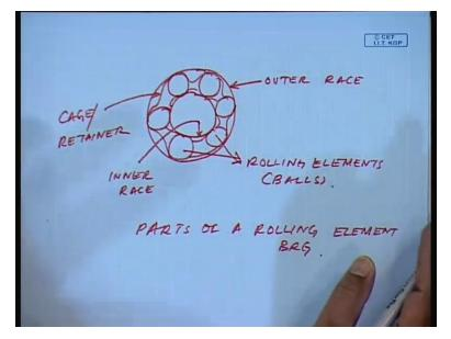
Let me just draw the bearing for all of you we have this so this is the outer race this is the inner race; these are the rolling elements or the balls. In this case and there is actually a cage or a retainer which are not drawn here which makes sure that this none of these two balls or rolling elements come in contact with each other? And this is known as a cage or sometimes known as a retainer part of a rolling element bearing.
