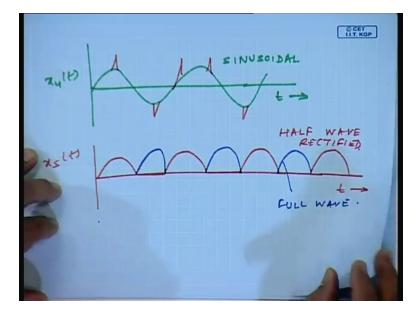
Of course this is the sinusoidal wave usually know when you are dealing with electrical signals of the constant frequency like a 50 Hertz signal, this is a sinusoidal wave. And you know you know in electrical equipment if this power supply is not a sinusoidal there are transients of kind of spikes etcetera in the signal they are known to; though their values will be less.
