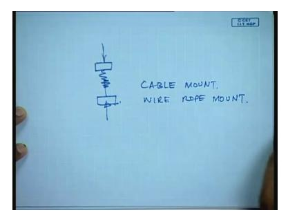
That the mount which we have is usually in one direction say okay. But suppose the motions are in three directions it becomes very cumbersome to put you know three Isolators in three directions rather the convenient way of doing it is through cable mount or sometimes in people also known as wire rope mounts. Because of the fact that there are no elastomers here, so they can be subjected to weather conditions.
