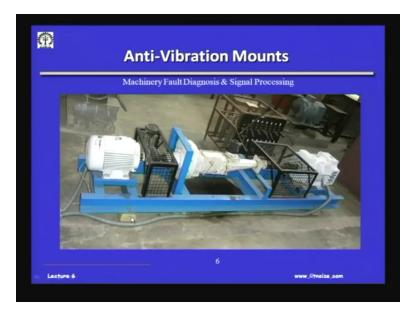
Another application or I should show you this anti vibration mounts, for example this is a set up from our lab. When you have the system running there will be lot of forces coming on to this structure. And this structure will eventually transmit to the foundation. So, these are what are known as anti vibration mounts. You can see one mount here, another mount here, so imagine if next to this machine, I had a very sophisticated laser based measuring systems okay.
