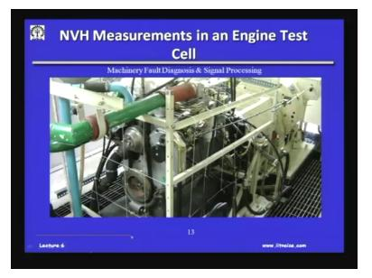
In closing this is one last slide wherein we will see the tuned dynamic sorry the torsional damper here on this engine and it will recall here in this engine we had done a lot of unconstrained layer damping to the oil sump to reduce the radiative vibration levels vibration and noise levels. This is actually in an engine manufacturers test cell we are doing the vibration study on the engine.
