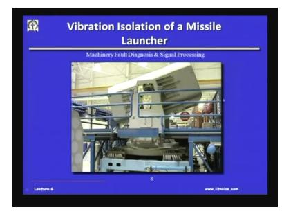
This is another case of a missile launcher and then here you see again the cable mounts have been put here and such a system could be put on the deck of your ship. Then once you have the missiles firing none of the motions are going to go through the deck to the other systems in the ship okay. Because you know you will see we will be doing some numerical, how to do we calculate the stiffness? How do we estimate the damping? How do you estimate the payloads of the mounts?
