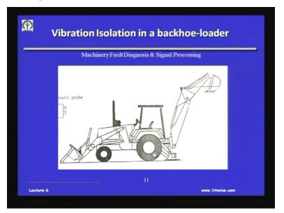
So, this is another example which I will use on a backhoe loader okay typically a backhoe loader or a truck. Essentially there are two strong components one in this engine and the chassis and if you observe and this is the unit where the operator or the driver sits and this is a cabin okay. And invariably now this construction equipment be it a bulldozer, be it loader they are always subjected to harsh vibrations because of the terrain.
