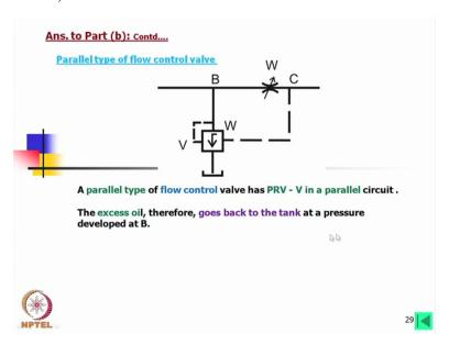
Now this is parallel type as you see there is no pressure control valve here. A parallel type of flow control valve has PRV in a parallel circuit. The excess oil therefore goes back to the tank at a pressure developed at B.
