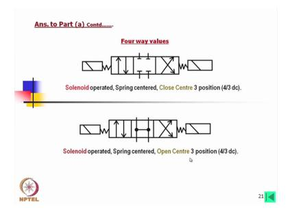
Now in case of 4 way valve, this is again solenoid operated spring centered again it is a closed centre 3 positions. So 4 by the 3 dc valve. Now again solenoid operated spring centered again open centre and 4 by 3dc valve.
