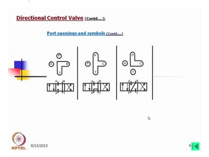
Now the last one valve like that possibly you can study of your own you can see this B to T is connected here P,C,T are connected and here this is P to B is connected.
