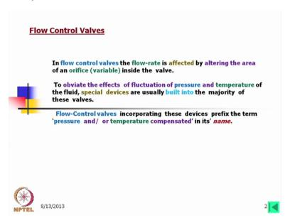
We shall discuss about flow control valves. In flow control valves the flow rate is affected by altering the area of an orifice inside the valve. The orifice is variable. To obviate the effects of fluctuation of pressure and temperature of the fluid, special devices are usually built into the majority of these valves. Flow control valves incorporating these devices prefix the term pressure and or temperature compensated in its name.
