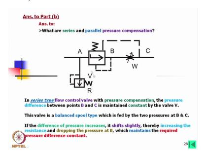
Now what are series and parallel pressure compensation? Now this is in series and there is a pressure relief valve and a series type flow control valve with pressure compensation, the pressure difference between points B and C is maintained constant by the valve V. if we adjust
