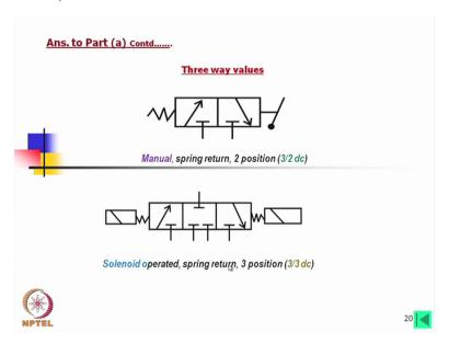
Now 3 way valves, 3 way valves means there are 3 ports. One side spring means again it is spring return and 2 positions. So 3 by 2 dc valve, there is no as such neutral positions either right side or left side. Now in this case, there is a neutral position. This is 3 position and solenoid operated. Here we should call the spring centre. So this is not spring return rather we should use the word spring centre.
