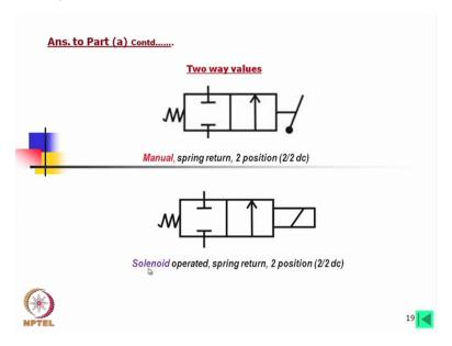
Now two way valves. This is a symbol of two way valves it clearly indicates this is a spring return and manual control 2 by 2 dc. Now here this is also 2 by 2 that is 2 way valves as well as it is 2 by 2 solenoid operated and spring return.
