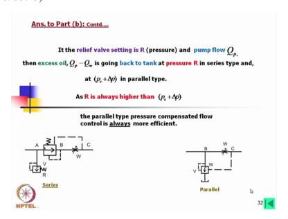
If the relief valve setting is R and pump flow is Qp, then Qp minus Qw is going back to tank at pressure R in series type. Whereas, it is going back to tank with only this pressure drop and this R is always greater than this. This means that in case of series connections, this bypass flow will
