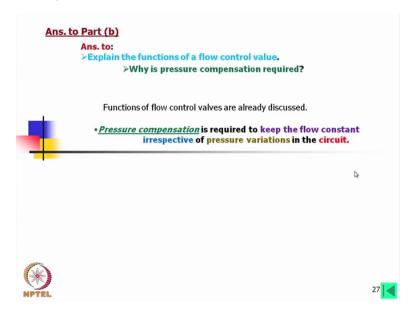
Now the answer to explain the function of a flow control valve. Why is pressure compensation is required? Functions of a flow control valves are already discussed. Now pressure compensation is required to keep the flow constant irrespective of pressure variations in the circuit. What we have discussed earlier while you are answering you have to write in this way.
