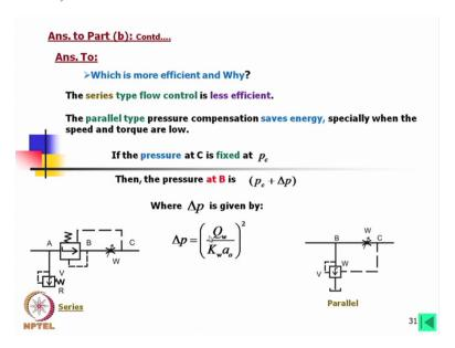
Now which one is more efficient? The series type flow control valve is less efficient. Here we have shown. The parallel type pressure compensation saves energy specially when the speed and torque are low. If the pressure at C is fixed at Pc then the pressure at B is Pc plus del p. where, del p is given by this equation.
