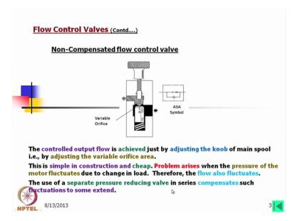
Now if we look into this figure, this is non-compensated flow control valve. This can work in both ways. This means in one way, it is a free flow through a check valve, but in other way it is
