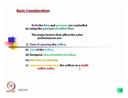
Now what are the basic considerations? First, both the flow and pressure are controlled by using the principle of orifice flow hat which I have discussed in lecture 4. The major factors that affect the valve performances are number one, rate of opening the orifice. Size of the orifice, here size includes the shape also. Third design characteristics orifice that also dependent on the shape of the orifice. Direction of opening. Sequence of opening the orifices in a multi orifice valve.
