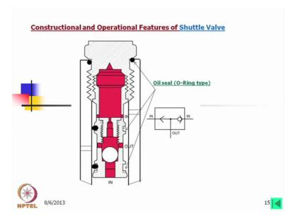
Now here are we are discussing some other valve also. This is constructional and operational feature of shuttle valve. If you remember this is the shuttle valve. What is the shuttle valve? In that case there are 2 inlets, one inlet here and another inlet here. Now whatever may be the inlet outlet is always through this. Now suppose there is a flow then simply this valve will go here and oil will go through this and it will go to the main system or may be to the drain.
