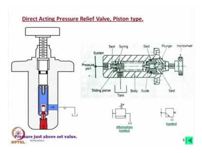
Now if I look into this colored figure. Now when the pressure below the set valve then as you can see that, this is the piston type and this is a another orifice. This orifice is put here, okay and then this is the piston and when there will be rise in pressure then it will open and oil will flow through this and it will go to the tank.
