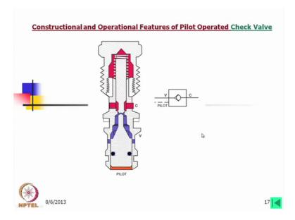
Now this is constructional operational features of a pilot operated check valve. Now in the case this is which I have described. The same thing in a colored figure as you see that oil is going through this and when it is going through, it can blow and it can go to the tank, but if the oil is coming from this side, it cannot go to the other side and the symbol is like this.
