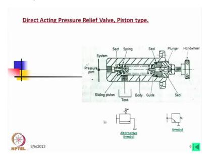
Now next one is the direct acting pressure relief valve, piston type. Again this is also direct acting, but instead of poppet or cone what we have used here a we have used a piston and if you look into this part, there is an orifice and which is giving a pressure to this piston which
