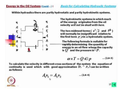
Within hydraulics, there are partly hydrostatic and partly hydrokinetic systems. If we consider a fluid power system usually you will find inside the pump performance, there is some part is hydrokinetic. Now once it is hydrokinetic means you have to consider the kinetic energy of the fluid that is velocity due to the velocity what is the energy of the fluid. On the other hand when we will reach into the hydrostatic parts we can neglect that part. We will consider only the pressure ports there.
