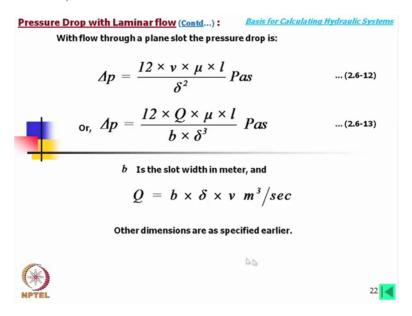
With flow through a plane slots the pressure drop is, now we have consider a slot. In that case, this is the slot height and then in terms of flow rate, this equation is converted into that and b is the slot width in meter and Q is given by this. That means here the area is b into delta. This is the slot height, this is the width, v is the velocity of the fluid.
