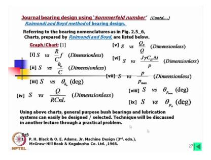
And you will find that there are chart available for S is a Somerfield number. This is dimensionless, R by C into f, R is the radius, C is the clearance and f. So you will get this chart from here we can calculate, f because R and C are known factor. S verses h0 by C that h0 is the gap at 0 position and that means directly towards the in the direction of load, then
