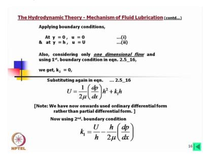
Now we apply the boundary conditions. Here the boundary condition is that when y is equal to 0, u is equal to 0 and at y is equal h, u is equal U, U means the velocity of the moving plate
