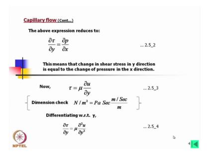
Now we can see that all terms will be cancel out except the terms these terms will remain there. So what we find that the change in shear stress. This is the shear stress change in shear stress in y direction is equal to the change of pressure in x direction. Now this is again the theory from the theory of shear stress and fluid. The shear stress is given by Mu del u del y
