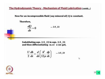
Now for an incompressible fluid say mineral oil Q is constant. Therefore del Q by del x will be 0 and the substituting equation 2.5-22 in equation 21 and then differentiating with respect to t, sorry with respect to x we get U by 2 del h by del x is equal to d by dx into h cube by 12 Mu dp by dx.
