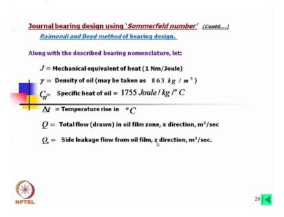
Along with the described bearing nomenclature, there are other factors also. J is the mechanical equivalent of heat and gamma is the density of oil, Ch is the specific heat of oil, Delta t is the temperature rise in degree centigrade, Q is the total flow in oil film zone, in x directions, Qs is the side leakage from flow oil film from oil film in z directions that is in the axial directions.
