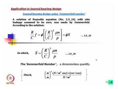
So now we if we consider the application in journal bearing design. Now Somerfield, he proposed that R by C f is equal to function of R by C square Mu n by p that is equal to phi into S. this means that this he this quantity he proposed which is defined by S and called as Somerfield number and it is a dimensionless quantity which can be verified from this. It is a dimensional quantity.
