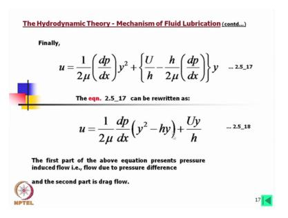
So finally we get you is equal to 1 by 2Mu dp by dx y square plus U by h minus h by 2Mu dp by dx into y, we can rearrange this and then we can write this equation in the form 1 by 2Mu dp by dx y square minus hy plus Uy by h. The first part now look into this equation, this first part of the above equation presents pressure induced flow clearly; this is a pressure induced flow. So this only will exist if there is a pressure difference and the second part is the drag flow.
