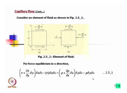
Now consider an element of fluid as shown in figure 2.5-2. Now this is the figure. What the element we have considered? This is a like a cube. The axis system is that along the direction of flow or along the direction of motion, the capital U is the plate velocity, small u is the fluid velocity in that direction capital U direction axis is x and along the h direction the axis is y and along that transverse directions there will be z axis okay.
