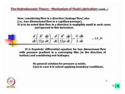
Now, consider the flow in z direction, we have consider along the peripheral direction of the hydrodynamic bearing. Now we are also considering the along the axis. Why it is important, because bearing will have certain length. So we must consider the equation also in the z direction. This means that if there is a pressure gradient in z directions there will be also leakage flow. Now the equation we will take the same form, so this is the full equation form
