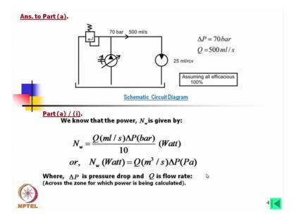
Now first of all we should draw a circuit like this. What is there? This is the variable displacement pump and this is the fixed displacement motor. Now obviously, this is a pressure relief valve. Here the pressure is mentioned and here, the flow rate maximum flow rate is mentioned. Now one thing is there we are using this term bar, but normally nowadays
