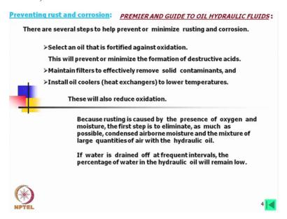
There are several steps to help prevent or minimize rusting and corrosion. These are select an oil that is fortified against oxidations. This will prevent or minimize the formation of destructive acids. Maintain filters to effectively remove solid contaminants and thirdly install oil coolers heat exchangers to lower temperatures, this is one important factor that due to the increase in temperature the many chemical processes are excited or may be those started with temperatures.
