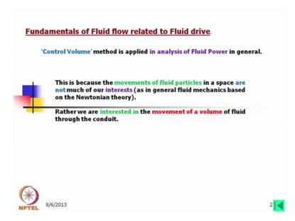
Control volume method is applied in analysis of fluid power in general. This is because the moments of fluid particles in a space are not much of our interests as in general fluid mechanics based on Newtonian theory. Rather we are interested in the moment of volume of fluid through the conduit.
