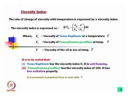
Now one important factor is the viscosity index. What it is? The rate of change of viscosity with temperature is expressed by viscosity index. It is expressed as the VIs subscript s is the
