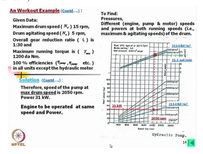
But actually if we carefully consider, we will find it will be 23 kilowatt what we have calculated in terms of flow and pressure, we as we have efficiency these results are coming in this way. Now therefore, speed of the pump at maximum drum speed is 2500rpm and it is 31 hp so this please note this correction. Engine to be operated at same speed and power so that is we have selected the engine like that.
