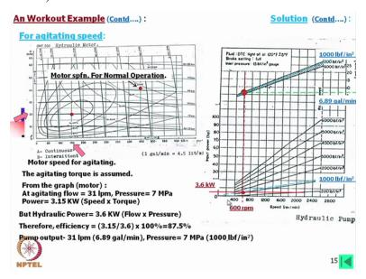
Now for agitating speed, say this this speed was as you see this is for motor specifications for normal operations, but for resulting speed what we found that 150 rpm and this is the torque
