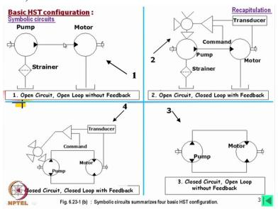
Now this is already we have seen, so this is open circuit open loop without feedback. Then we can have the open circuit closed loop with feedback so there is a feedback so this means that depending on the output of the motor this pump can be controlled, so this is open circuit closed loop. Similarly we can have the it is a closed-circuit but open loop and finally we can have closed-circuit close loop with feedback that means this is not only closed-circuit as well as closed loop.
