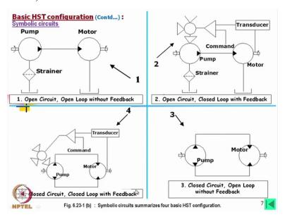
Now, if we try to understand through this symbolic representation, we see that this is a unidirectional pump and this is a unidirectional motor, they are simply connected like this and oil is from the reservoir and oil is going back to the reservoir. So we should consider this definitely open circuit and also it is open loop without feedback, no control is there so this is open circuit and open loop.
