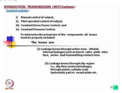
Now control system may be manual, control pilot operated control, constant horsepower control and constant pressure control, anything you can achieve, you can design the system like that. To
