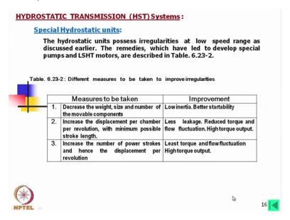
Now we can also go for special hydrostatic transmission unit, which that first of all what we should do? Decrease the weight, size and number of the movable complaints, so low inertia, better start ability. And increase the displacement per chamber per revolution, this is the leakage loss, reduced torque, et cetera. Increase the number of power strokes and hence the displacement per revolution, so least torque and flow fluctuation, high torque output.
