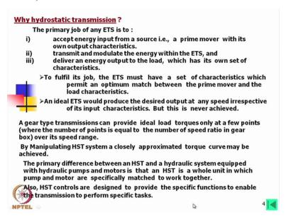
Primary job of an energy transmission system is to; except energy input from a source that is a prime mover with its own output characteristics, look at this. We are using a pump, we are using a motor for the hydrostatic transmission system, but when we are thinking of driving this pump that is having its own characteristics. So and our output will have it needs its own characteristics, so 1<sup>st</sup> of all from the prime mover to the output we have to match that characteristics. Now
