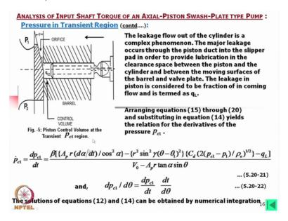
The leakage flow out of the cylinder is a complex phenomenon. The major leakage occurs through the piston duct into the slipper pad in order to provide lubrication in the clearance space between the piston and the cylinder and between the moving surface of the barrel and valve plate, the leakage in piston is considered to be fraction of incoming flow and is termed as q L, okay we must now consider the total leakage q L.
