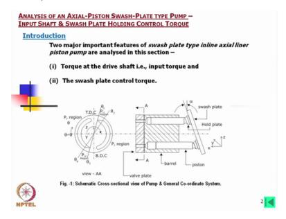
The major important features of swash plate type inline axial linear piston pump are analysed in this section and we consider the torque at driving shaft that is the input torque to drive the pump and the swash plate control torque. Now as we are rotating the barrel and it is there is a suction and compression of oil definitely we need to supply some torque depending on the pressure.
