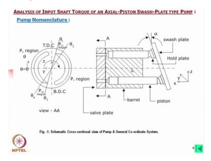
Now looking into this pump I think next which can go into the next slides and here let me explain the components and the valve angles. Now this is already described this is barrel, this is piston and this is the here it is not very clear but this is the slipper pad and there is another holding plate which is holding all these pistons together simply a plate which is again placed between this valve plate and the swash plate by a spring.
