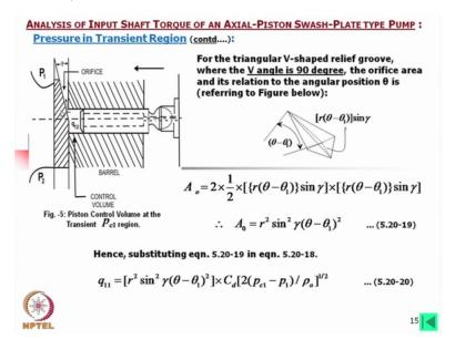
For the triangular V-shaped relief groove, where the V angle is 90 degree, I am showing this figure now which is 90 degree, this angle that means this angle is consider 90 degree this angle is 90 degree, okay. The orifice area and its relation to the angular position theta is given by we consider let us see this angle say this angle must be theta minus theta 1, theta 1 remember this is not for the piston one but for the region on the valve plate we have shown.
