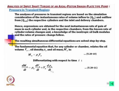
The analysis of pressure in transient regions are based on the simulation considering the instantaneous rates of volume inflow Q 1 and outflow from the respective cylinders and the yielded and delivery chambers. Hence, expressions are obtained for the next instantaneous rate of gain of mass in each cylinder and with the respective chambers form the known rate of cylinder volume changes and a knowledge of isentropic oil bulk modulus and the rates of pressure change follow.
