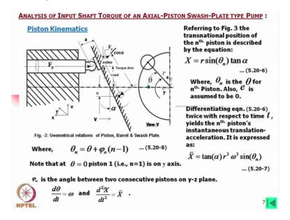
Now referring to figure 3 the translational position of nth piston is described by the equation which we have done also earlier we can write down this equation X at an instant is equal to r sin theta into tan alpha and then so theta n is theta for nth pistons also e is assumed to be 0 here look at this figure in this figure what we have shown that as if this pivot point is not intersecting this axis that means pivot of the pivot point of the swash plate is not on the axis of the drive shaft.
