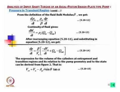
From the definition of fluid bulk modulus this can be beta can be expressed again in this form, okay this we have in earlier lecture I have shown. Then from the continuity of fluid flow we would write these equations remember this we have consider at an instant that means when we are considering these equations definitely for that time that pressure and temperature are not varying or there effect is negligibly small.
