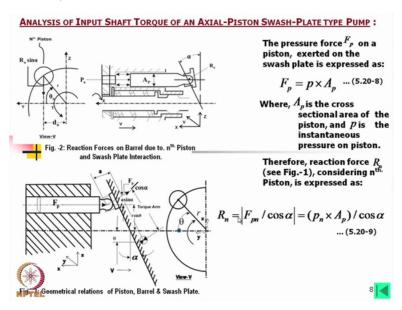
Now what we would consider we will simply calculate what is the F p what is this force F p is the force acting over there on the pistons here here it is shown this is the F p, F p is nothing but the p into A p. Now again here we have kept the p general but in case of nth piston we have to (push) put p n into A p because for a pump A p will given constant. So the force can easily be calculated from these equations.
