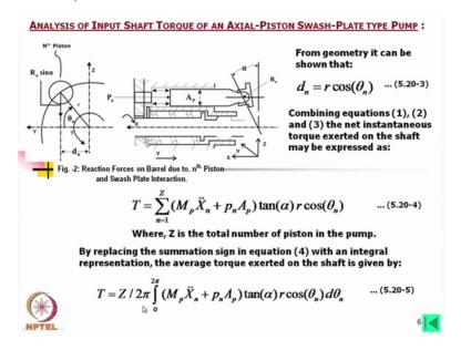
Now from geometry it can be shown that this distance is r cos theta n, okay this is r and cos theta n is the at an angle of nth piston so easily we can calculate what will be the torque arm. Combining equations 1, 2 and 3 the net instantaneous torque exerted on the shaft may be expressed as this is we have consider all the pistons which are giving the force. Now look at this in this case we have consider n is equal to 1 to Z and we have taken this summation of this.
