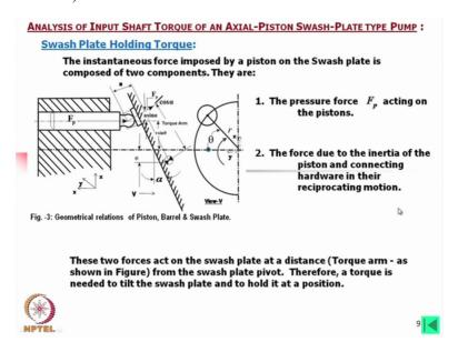
Now the instantaneous force imposed by a piston on the swash plate is composed of two components again. The pressure force F p acting on the pistons and the force due to the inertia of the piston and connecting hardware in their reciprocating motions which we have already shown. Now we are calculating trying to calculate the swash plate holding torque. Now look at this figure you see this is the force acting on the pistons.
