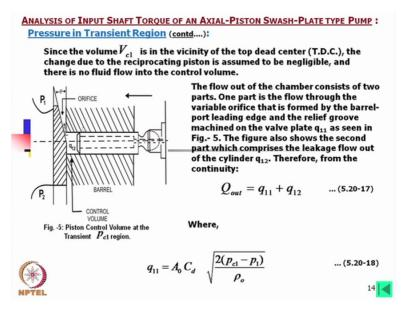
Since the volume V c1 is the vicinity of the top dead center remember what is top dead center and bottom dead center, V c1 is in the top dead center that means which one fully open ya no this is top dead center means fully closed one this smallest volume, V c1 is the vicinity of
