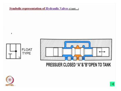
However, before that we should consider the other type valves. There are other options also. In this case, as we see that at neutral position P is closed, but all other are connected tank. Now as you move in this directions P will be connected to B, A will be A will still remain
