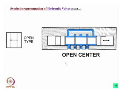
Now if we consider the open center, you can see just this spool is changed. In this case, the P is connected to the all ports at this neutral position. Now if I move this in the right or directions then P will be connected to B and A will be connected to tank and if I move in the other direction, it will be reverse.
