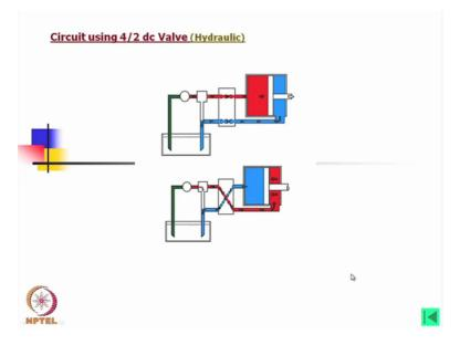
Now this is a very simple circuit is shown with a direction control valve. This is as if on-off not on-off type. This is two positions you can say either it is going straight or it is going in the opposite directions. So this circuit to understand the operations we can present it like this, but for general purpose we will use the some symbols.
