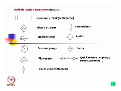
Now symbols for basic components. So this is a reservoir and we find another line here, which is baffle. What it is there? The oil main oil will come here or may be the return oil is coming here. Then this will go over this with some contamination will be can kept here as well as the foaming foam inside will be reduced. So baffle are was used. So that details you can learn from any book we shall not discuss much more on this how the tank is constructed.
