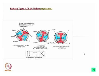
Now if we look into this. This is 4 by 3 dc valve, but this is a rotary type. These are not normally used, but still at one point this valve be can popular. In comparison to this the spool valve has better leakage property that means this leakage with that spool valve. Here it will be more leakage, but if this is easy to operate.
