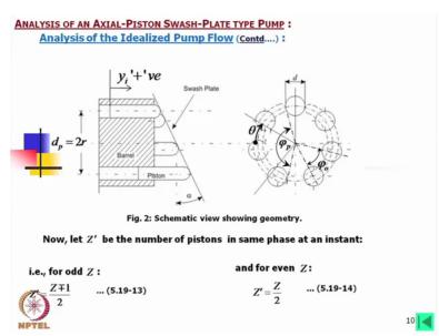
Now we consider Z dash be the number of pistons in same phase at an instant that means Z dash is equal to null, Z plus 1 by 2 or Z minus 1 by 2 in case of odd number, in case of even number this is simply Z by 2. Here I have expressed, okay so for even, odd number and even number we expressed in this way.
