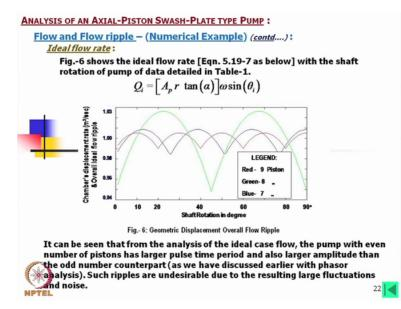
And then for that we have plotted these equations, look at this for 9 pistons the ripple is coming like this please note that we have considered the overall volume displacement is same displacement we have not mentioned the diameter of the pistons. So therefore what we have considered from the average flow is same considering that for 9 pistons you can see what are the ripple and for 7 pistons the this one is the 7 pistons for blue one but as you see for the 8 pistons it is increasing.
