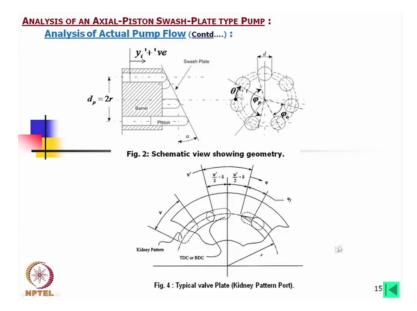
Now how it is varying, here this is the port we have shown the manifold this is actually continuous, on the barrel we could leave this hole as a bore equal to the diameter of the piston that means this could be made through hole but you will find normally this hole the cylindrical hole upto almost upto the end but end is not the cylindrical hole instead of that there will be a small kidney port, this is kidney pattern it is written kidney pattern usually it will be of this shape.
