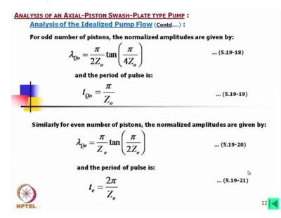
Now this two expression here the amplitude similar way we can define the amplitude in this way and the period of pulse is Pi by Z 0 this is of course for the odd number of pistons. For
