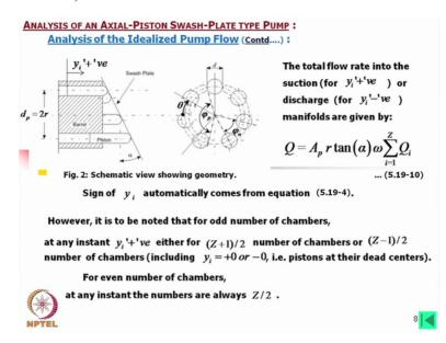
Now the total flow rate into the suction thus y i is positive or discharge y i is negative manifolds are given by the same equations will be same because this we are only this defining the quantity but we have to consider for y positive and y negative separately because if we integrate together ultimately it will become 0 because one is in positive and other is in negative so that consideration we have to make but if we do it then this will be the expression.
