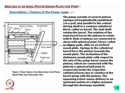
Now this pump such pumps it is widely used it consists of several pistons equispaced longitudinally equidistant and parallel to the central driving shaft in a common cylindrical block called as barrel. Now this one is the barrel, this is the drive shaft and these are the pistons, these pistons are led on a pitch circle diameter and angle between two pistons are constant also, okay.
