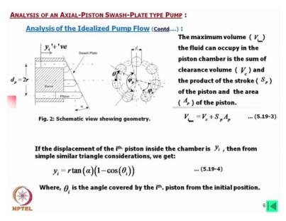
The maximum volume V imax the fluid can occupy in the piston chamber is the sum of clearance volume we will consider now there is a clearance volume and the product of stroke of the pistons and the area of the piston this means if A p is considered as the area of this piston this diameter is d that means Pi d square by 4 is equal to A p so A p into stroke length
