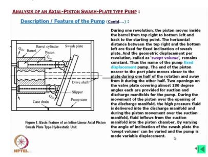
Now during one revolution, the piston moves inside the barrel from top right to bottom left, top right means this is as it is in the right side we are saying top right and to the left. The horizontal distance between the top right and the bottom left are fixed and fixed inclination of swash plate this means if we increase this inclination this length will increase that movement will increase which is called stroke length, the stroke length will increase.
