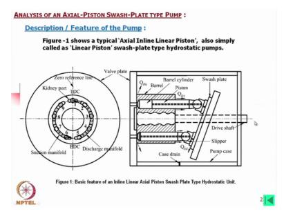
Now I would like to mention that I have written here hydrostatic pumps I have mentioned hydrostatic pumps but basically we call it rotary hydrostatic units which includes pumps and motors, we shall describe a pump, we will analyse a pump here. However, the analysis for the motor will be more or less same considering their flow pressure, etc. Now here in figure 1, what I have shown a typical axial inline linear piston which is simply called as linear piston swash plate type hydrostatic pumps.
