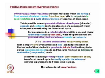
Positive displacement machines are those machines which are having a fixed amount of volume transfer from flow input side to output side in each revolution or a cycle of linear motion, irrespective of their speed. This means that whatever will be the geometric displacement the same amount will be transferred from input side to the output side let it be a rotary machines or a linear actuator this is of course there is no leakage we are considering there is no leakage.
