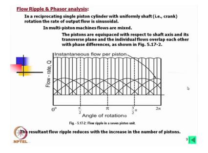
In a reciprocating single piston cylinder with uniformly shaft crank rotation the rate of output flow is sinusoidal. In multi-piston machines flows are mixed that has to be here I would like to mention that as flows are mixed we call it DC direct current we can compare with it is a DC type machines, whereas there is also possible we can make alternative flow hydraulic machines.
