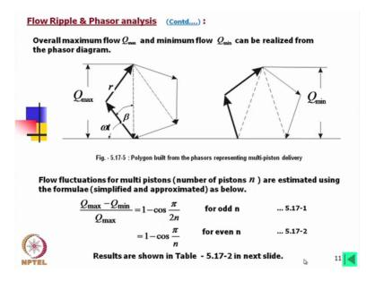
Overall maximum flow Q max and minimum flow Q min can be realized from the phasor diagram, it is like that. Say we have five pistons, so what we can do this phasor say this is with respect to the shaft this is the first piston position, the second piston obviously you will find it will be here because this angle difference will be say if this is 0 plus omega t, then this will be 0 plus 2 Pi divided by 5, we have 5 pistons plus omega t.
