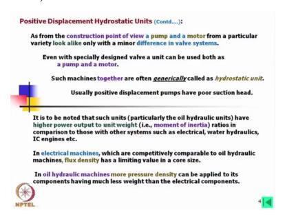
As from the construction point of view a pump and a motor from a particular variety look alike only with a minor difference in valve systems. It is very difficult to identify whether it is a motor or pump, in case of pump we rotate the shaft and oil is taken in in suction stage and it is delivered at compression stage, in case of motor it is reversed the high pressure oil is pumped in and then output is taken through the shaft.
