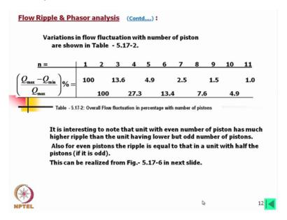
And this we have presented here in this table. Now if I consider 1 pistons then Q min is 0 in the flow ripple that it has will be 0 definitely, okay and so this will be 100 percent, 100 percent fluctuations that means if you consider the sinusoidal curve it will be from the top to bottom at the 0 lying so this is 100 percent and if we look into this formula this is quite interesting that for 2 pistons also it is 100 percent.
