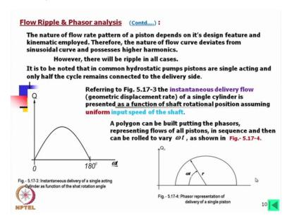
The nature of flow rate pattern of a piston depends on its design features and kinematic employed. Therefore, the nature of flow curve deviates from sinusoidal curve and possesses higher harmonics, which I have explained. However, there will be ripple in all cases whatever may be the harmonics are there, there will be ripple. It is to be noted that in common hydrostatic pumps pistons are single acting and only half the cycle remains connected to the delivery side.
