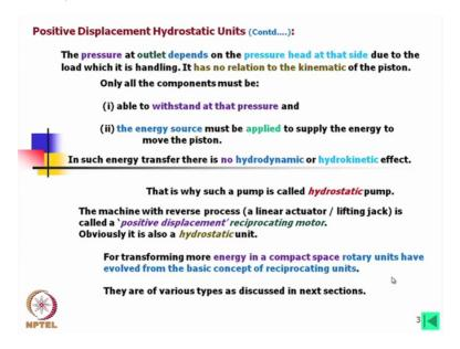
The pressure at outlet depends on the pressure head at that side due to the load which it is handling. It has no relation to the kinematic of the piston, this means that if there is no pressure or if it is not transmitting any load only the pump in the volume you may find there is no pressure on the oil except it has to overcome some resistance so there will be some pressure.
