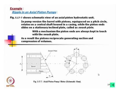
Now we are considering for the ripple we are considering an example now this is what we have shown that is axial piston pump how it works? We will come into detail later but let me explain a little bit this is called a barrel, barrel means it is just a cylindrical body of thickness of this much and then there are holes, how many holes that depends on how many piston we are using, you can see here you have used 7 pistons so there are 7 equispaced holes on which the pistons are placed.
