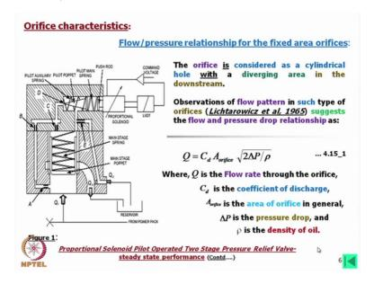
Now flow pressure relationship for the fixed area orifices again we consider A and B, the orifice is considered as a cylindrical hole with a diverging area in the downstream. Actually these orifices are like that almost straight hole is there but at this side I mean in towards the downstream side this is upstream if the flow is going like this this is upstream, this is downstream slight divergent is there.
