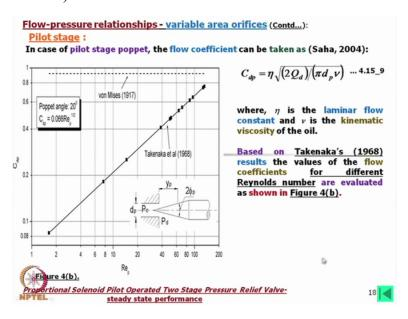
Now for the pilot stage similarly this formula can be used and it is called laminar flow constant and this is the kinematic (kinetic) kinematic viscosity sorry not kinetic, kinematic viscosity of the oil. Now in this case I think I have made mistake here 1 by 8 this relation will be more or less same and he also proposed this formula for this one this formula but in this case as you see for the pilot stage this curve is different from the main stage. In this case this angle is very low.
