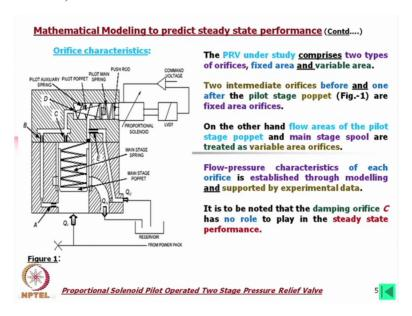
Now first of all we shall look into the orifice characteristics. Now again coming back to the this valve then A, B, C, E these four orifices apparently it is we should call the short tube orifices. Now in broadly we should say this comprises this valve will comprises of two type orifice one is that fixed area 1, 2, 3, 4 the fixed area orifice and the other is variable area this is one variable area here, another variable area is there.
