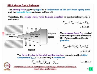
Now pilot stage force balance can be achieved by this, this is the pressure force and this is the driving force and this equation can be written in this form, this F Dr is the driving force, here what we find the auxiliary spring force and then flow force and this pressure force these three forces are flow force, spring force and the pressure force, okay. Now the pressure force is
