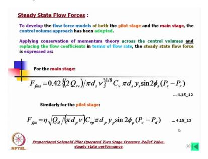
Steady state flow forces model for both pilot stage and main stage the control volume approach is adopted. Now we have to find out the flow forces. So main stage flow forces can be expressed like this, this is again using the flow force equation we have arrived into that but I think we need to explain this in a little better way so maybe we shall continue in the next day.
