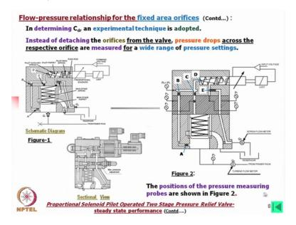
Now in determining C d an experimental technique is adopted. Instead of detaching the orifices from the valve, pressure drop across the respective orifice are measure for a wide range of pressure setting. You see if we use this orifice separately we can it is possible that (())(32:01) can be made and there the orifice can be put and we can find out its C d but instead of that we have used all the orifices in their positions and then we have measured pressure, how?
