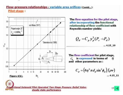
Now the flow equation for the pilot stage, after incorporating the functional relationship of the flow coefficient with Reynolds number yields if we use all such formula then we can put in this form and the flow coefficient of the pilot say C p is expressed in terms of Eta and other parameters as this we can use this formula there, okay so now we can use this formula to flow through this.
