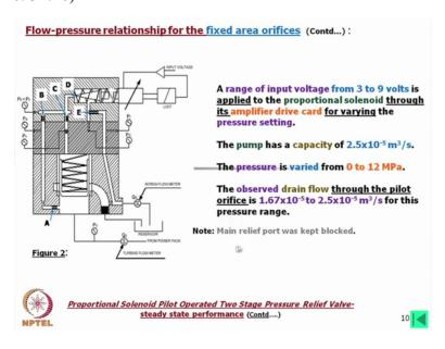
Now so what we find these are the orifice this we want and these are the pressure transducer and then a range of input voltage from 3 to 9 volts is applied to the proportional solenoid
