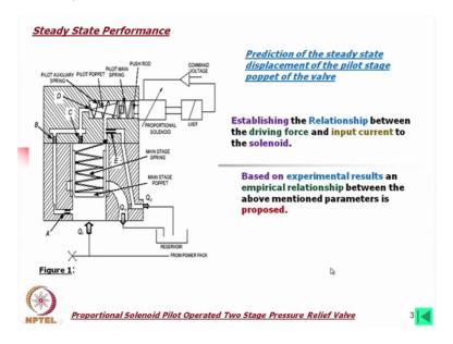
Now we will predict we will try to predict the theoretically what will be the steady state displacement of the pilot stage poppet of this valve. Now establishing the relationship between the driving force and input current to the solenoid in this case we have consider the current is the input input current to the solenoid. Based on experimental results an empirical relationship between the above mentioned parameter is proposed.
