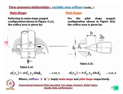
Then main stage you can see this I have mentioned this all this angle this is the main stage for which we can write down this formula and similarly for pilot stage we can write down this formula, this formula is same only this subscripts that s is for the main stage and p is this for pilot stage but you should remember these two angles are different so definitely nature of variation of this area with this stroke definitely or stroke or displacement will be different.
