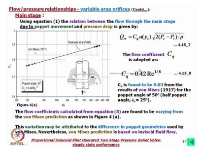
Now flow pressure relationship variably orifice, main stage it can be written in this form. The C q is the flow coefficient, now here instead of coefficient of discharge we call it flow coefficients and C q can be written in this form, where Re is the Reynolds number 0.42 like this. Now this is also established experimentally but if we now compare with the Von Mises
