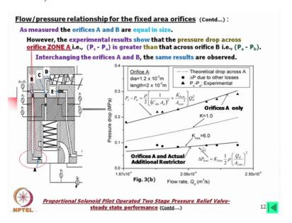
Here I have mentioned that as measured that A and B orifices are equal in size. However, the experimental results show the pressure drop across orifice zone A here is greater than that across orifice B that means here it was more pressure drop this means that there are more restrictions I would like to mention there is no way to verify what is there although you see this construction wise here there was a hole but that hole was blocked and neither we
