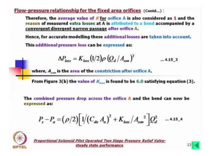
Now average value of K for orifice A is also considered as 1 and the reason of measured extra losses at A is attributed to bend accompanied by the convergent divergent narrow passage after orifice A. Hence, for accurate modelling these additional losses are taken into account. This additional pressure loss can be expressed as with this formula K loss half Rho Q d A con that area of that restriction to the power square.
