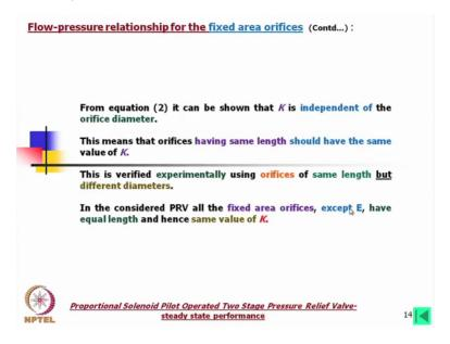
Now from equation 2 it can be shown that K is independent of the orifice diameter, this is another thing that K is not dependent on diameter it is dependent on the length this means that orifices having same length should have the same value of K. This is verified experimentally orifices of same length but different diameters, we further conducted the experiment by using those orifice changing the diameter of the hole keeping the length same and we found this K value is coming same.
