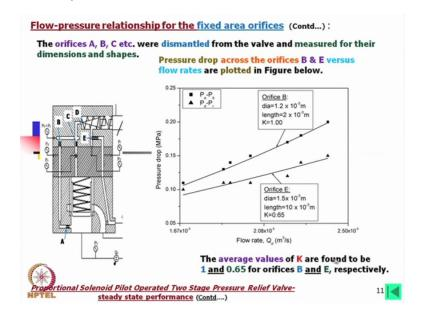
Now A, B, C etc were dismantled from the valve and measured their dimensions everything were measured. Pressure drop across the orifice B and E you see that across the B and E flow rates are plotted in this figure, if we look into this, this is the orifice E and this is the orifice B, okay. Now here one interesting point is that we found that E is having a different dimensions then B however, A was having the same dimension what in B.
