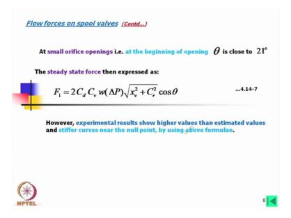
A small orifice opening at the beginning of valve opening we should say valve opening theta is closed to 21 degree which I have shown if you observe while the valve is opening jet angle is almost 21 degree this is of course for the rectangular port. Now then for that this F 1 can be expressed like this, this is again not we are not considering the direction but the magnitude can be taken like this, where cos theta can substitute 21 degree.
