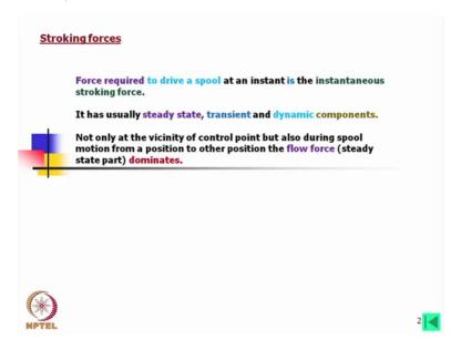
Force required to drive a spool at an instant is the instantaneous stroking force. It has usually steady state, transient and dynamic components. Not only at the vicinity of control point but also during spool motion from a position to other position the flow force which is and steady state part of flow force dominates.
