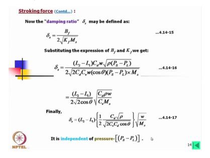
Now the damping ratio del s may be defined as B f by K f M s, this is also standard it is called damping ratio. Now this damping ratio we can substitute these two in this equation and we can find that damping ratio is expressed by L 2 minus L 1 C d w under root Rho P s minus P L and in the denominator 2 root over 2 C d C v w cos theta P s minus P L into M s, okay that also can be calculated because all data will be known something we can measure and rest of the part we can calculate.
