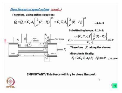
Now what we can write so we now use orifice equation and we can write Q 1 is equal to Q 2 because this is same, this is coefficient of discharge into A 0, A 0 again I am considering the area for the orifice area has open, then 2 by Rho P 1 minus P 2, P 1 is the pressure inside, P 2 is the outside of this orifice this if you remember the figure. Now this is again we are resolving into C c and C v, the contraction coefficient and velocity coefficient, okay.
