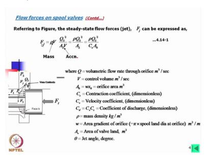
Now referring to this figure the steady state flow force that is jet, F j can be expressed as, this is Rho into V the V is the velocity of the fluid and then Q 2 square is the flow rate divided by
