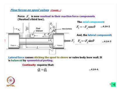
Now force F j we will now resolve into two components one is the direction of the axis F 1 and another is F 2, the axial component F i can be written as F j cos theta, why it is minus it is if we resolve this force that will have the component in this directions but this is we are considering what will be reaction due to the jet force so the minus sign is coming over there. So clearly this will be F j cos theta.
