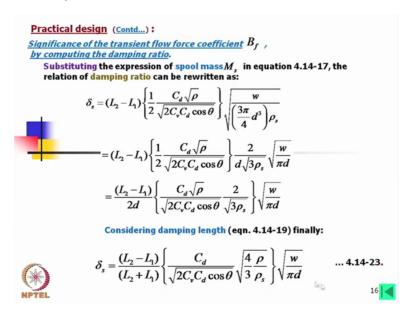
Significance of transient flow force coefficient B f that is the damping coefficient by computing the damping ratio substituting the expression of spool mass M s in equation 17, the relation of damping ratio can be rewritten as look into this we have now put this mass and we have rewritten this damping ratio which we can equate to this value, okay.
