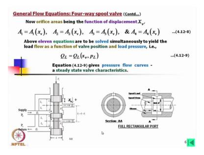
No orifice areas being sorry now orifice areas being the function of displacement x v what it is this area basically that opening into the displacement will give the area of this orifice. So what we write A 1 the area which we have consider in the equation is A 1 x v actually it is function of x v. Similarly A 2 is equal to A 2 x v, A 3 is equal to A 3 x v and A 4 is equal to A 4 x v, okay.
