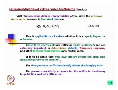
With the preceding characteristics of the valve the pressure flow curve becomes in linearized form as del Q L is equal to K q del x v plus K c del P L that P c is the flow gain and pressure strength sensitivity. In this term we can write down the equation that means if these two values are known for a valve if the valve characteristics are fully defined in a operating zone, that means for each and every operating zone you should have this values available in your hand.
