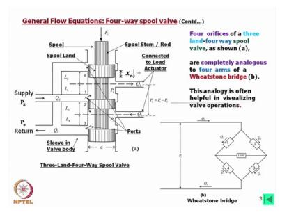
Now look at this figure what we see that this is Three-Land-Four-Way Spool Valve, if we look into the spool it is having it is put inside a sleeve which is which again inside the valve body say this portion other than this spool we can say this is a integral body you can say inside the spool can move, this you may consider as a sleeve inside the valve. Now here I
