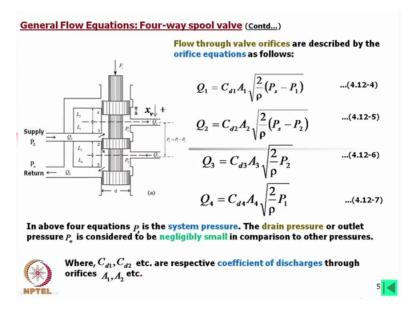
Now this here I have shown that valve displacement x v and this is the positive direction we have considered the positive direction along the direction of the force being used force F 1
