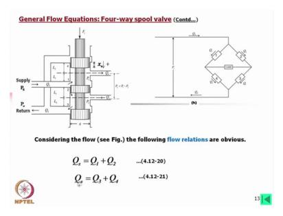
Considering the flow the following flow relations are obvious that Q s is equal to Q 1 plus Q 2, Q s is equal to Q 1 plus Q 2 and Q s is equal to Q 3 plus Q 4.
