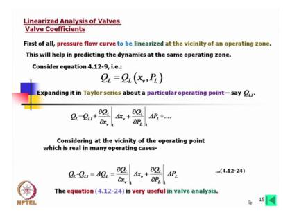
Now here to get the results I mean how much force is required, what will be the transient, etc we should use some more useful coefficients, what are these? First of all pressure flow curve to be linearized at the vicinity of an operating zones, we have shown that pressure flow curves which is equal to Q L is equal to Q L is a function of x v and P L that equations. So we now expand that equations and we will find that how it can be solved.
