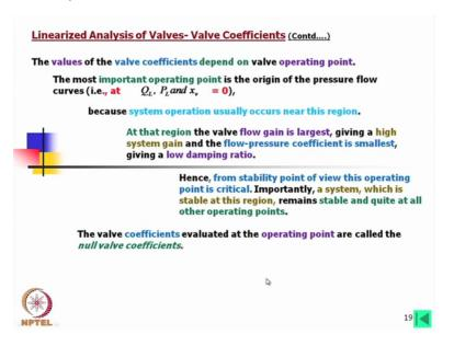
The values of the valve coefficients depend on the valve operating point, that I have mentioned this will vary different point. The most important operating point is the origin of the pressure flow curves, why it is most important? Usually what we need that a load has to be made in one direction and next movement it has to move in the other direction also so definitely operating point near the null point is most important, okay.
