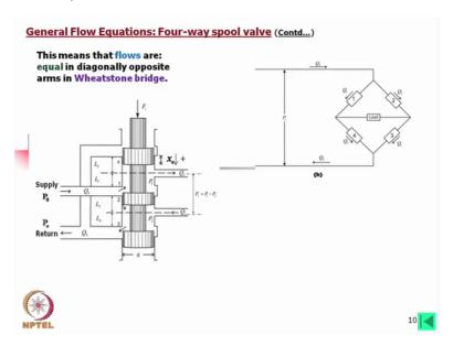
Therefore we can say this means the flows are equal in diagonally opposite arms in Wheatstone bridge. This is equal and this will be equal, okay.
