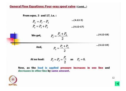
So from equation 3 and 17 these two equations we get two very important equations that P 1 will be always equal to P s plus P L by 2. Now here again I would like to mention we have taken Four-way three lands spool valve, these are matched and symmetric and in that case what we find P 1 is equal to P s plus P L by 2 that is why I told that if system pressure is 10 Mega Pascal other one will be half of that to get this value, you can equate like this.
