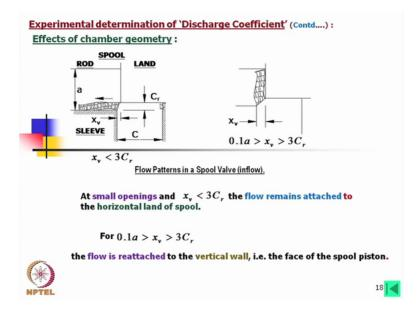
Now in this case if this spool displacement is less than three times the clearance then the flow remains attached to the horizontal land of the spool (sorry I think here I have made a mistake) it is horizontal land of the body. Then if it is 0.1a within this range less than 3 of the radial clearance but higher than 0.1, of sorry it is less than this but higher than 3C r, in that case we will get that reattached to the vertical wall, of the face of the spool pistons.
