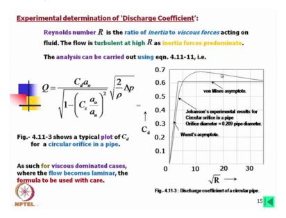
Now Reynolds number is the ratio of inertia to viscous forces if you remember the formula this will be definitely inertia by viscous forces acting on the fluid. The flow is turbulent at high Reynolds number as I told if the Reynolds number is high in that case it becomes turbulent that means in many cases in the orifice flow you will find the after the orifice the flow is turbulent.
