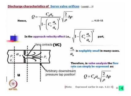
Now we have replaced C v into C c with C d, so this has come into this form. Now in many cases you will find that this quantity a 0 by a u is very I mean a u is very high in comparison to a 0. So totally this quantity becomes very small and we can in most of the cases we can neglect this part or this means that we can consider this part as 1, this part is equal to almost 0 and this is 1.
