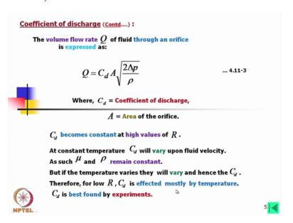
Now again we have written the a 0, a 0 is the normally the geometric area. Now the volume flow rate Q of fluid through an orifice is expressed as Q is equal to C d A (by twice) under root twice pressure drop 2 into pressure drop divided by Rho this is very known formula widely we use but this I have again used to concentrate on the C d the coefficient of discharge factor.
