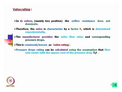
Now first of all we learned about what is valve rating? In dc valves, mainly if we consider two positions the orifice resistance does not dominate. This means that usually for direction control valve which we should consider as a on of valve, the orifices are not so accurately made although it is made close centre or open centre that means overlap, under lap or evenly it is made critical centre but orifice edge finishes or tolerances are not that close.
