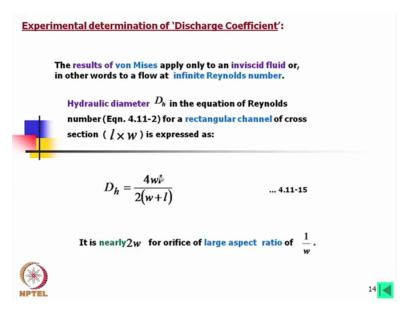
The results of von Mises apply only to an inviscid fluid, now again this is a inviscid fluid you can understand that with the viscosity definitely it changes, I mean he developed this model for inviscid fluids, okay. In other words to a flow at infinite Reynolds number that means (very) this is applicable model is applicable where the Reynolds numbers are high we should take these words to this meaning, okay.
