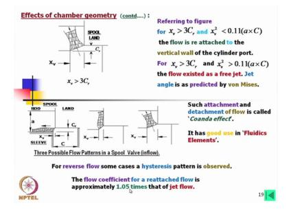
Then if it is slightly higher say if this X v is 3 times the clearance that is the spool displacement is 3 times the clearance and also this condition is satisfied you can see these conditions this is in the ratio of a into C is this distance a is this distance then in that case flow is re attached to the vertical wall of the cylinder port, whereas if this is satisfied but this value is greater than the 0.11 into a into C the flow existed at free jet. Jet angle is predicted by von Mises, okay.
