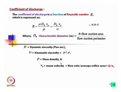
Now the important factor coefficient of discharge again the problem main problem is that in a valve the coefficient of discharge is an important factor to calculate many properties of the valve. Now coefficient of discharge for a valve for whole range may not be given, so we have to look into this how much this coefficient of discharge vary within the range of this valve and some data will be given there from which we can reassess what will be the coefficient of discharge.
