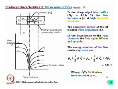
Now to find out a discharge characteristics of a servo valve orifice, you see this look at this orifice in a pipe you must have learned already how to find out this coefficient of discharge Vena contracta in may be in the hydraulics classes, one important thing is that always you will find that orifice usually this orifice is surface. You will find that at the entry point the diameter is the lowest, area is the lowest and a 0 is the area, the a 0 (())(26:08) mentioned.
