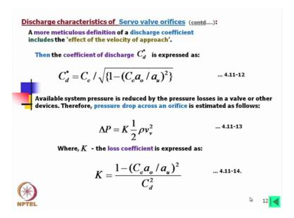
A more meticulous definition of a discharge coefficient includes the effect of velocity of approach. So for more accurate calculation to characterize the servo valve we need to consider this part. So therefore the coefficient of discharge that C d star is expressed as C c divided by 1 minus C c a 0 a u whole square. Now in this case that I would say that the C v
