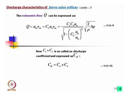
Now the volumetric flow Q can be expressed in this form if we remember the earlier equations then we can rewrite this equation in this form, okay. So here we are getting the C c into C v which is called the discharge coefficient and expressed as C d is equal to C c and into C v. Now this is this already you know but still it is explained here how we have arrived into this.
