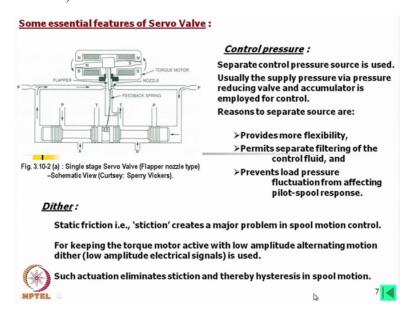
Then we think of this control pressure. Now separate control pressure. That means this source is a separate source not the main source here. Usually the supply pressure via pressure reducing valve and accumulator is employed for control. Reasons to separate source are one, provides more flexibility, secondly permits separate filtering of the control fluid and thirdly prevents load pressure fluctuation load pressure fluctuation from affecting the pilot spool response.
