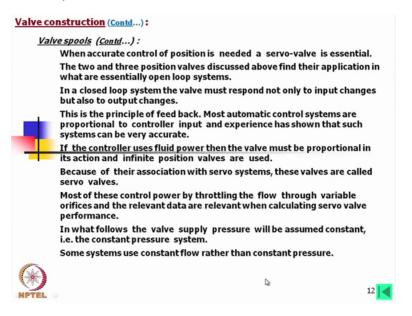
Now valve spool when accurate control of position is needed a servo valve is essential. The two and three position valves discussed earlier find their application in what are essentially open loop systems. In a closed loop systems the valve must respond not only to input changes but also to output changes. This is the principle of feedback, most automatic control systems are proportional to controller input and experience has shown that such systems can be very accurate.
