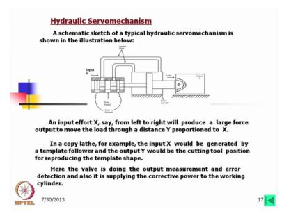
Now we can think of the servo mechanism, which is also with hydraulic. The servo term as you know, it is feedback control of motion and position. So a schematic view is shown here.
