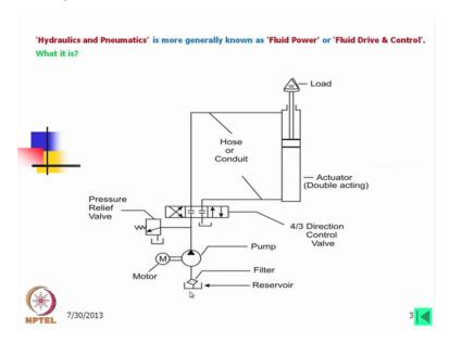
Hydraulics and pneumatics is more generally known as fluid power or fluid drive and control, but let us know what it is. Consider a load which is to be lifted to a height. There are many other mechanical means, but we can think of an actuator which is piston cylinder, we can put it vertically and on the piston end and we can put the load, which can be lifted by means of lifting the piston through fluids.
