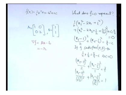
In our previous lecture, we introduced the concept of the gradient search based techniques, and we tried to illustrate one of those methods with the help of an example. So, we will continue with that example. So, in the example, our objective was to solve the system of equation A x equal to b, where A is given by this matrix, and b is given by this vector. So, what we first did is, we first obtain f(x), which is half of x transpose A x minus b transpose x plus C.
