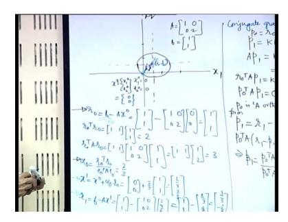
So, the same example, where we have A is equal to  $1\ 0\ 0\ 2$ , and b is equal to  $1\ 1$  you have to find out the value of x. So, remember that the first few steps of the conjugate gradient method are same as the first few steps of the steepest descent method, up to
