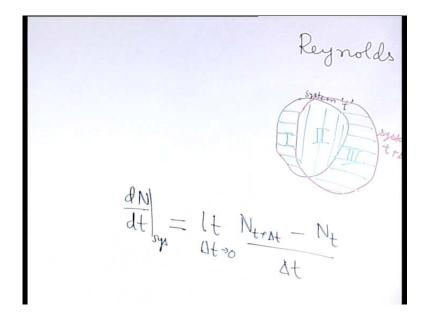
N at time t plus delta t is N at 2 at time t plus delta t plus N at 3 at time t plus delta t. We are interested to find out what is dN dt of the system; that is, the rate of change of N for the system. So to do that, we can write dN dt of the system is equal to limit as delta t tends to 0 N at t plus delta t for the system minus N at t divided by delta t.
