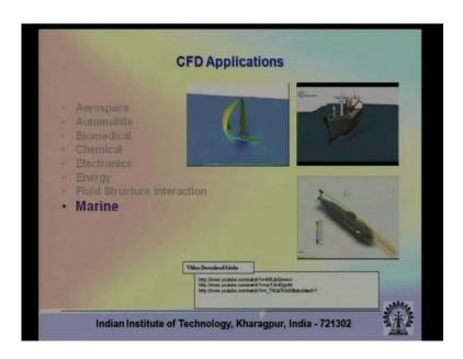
CFD has lots of applications in larger scales also, like marine applications. So, you can have a flow past ships and boats and even submarines, and though these are of much larger length scales than many of the examples that we have seen till now, but like these are still very important, and huge component of the marine design now these days relies on the use of CFD.
