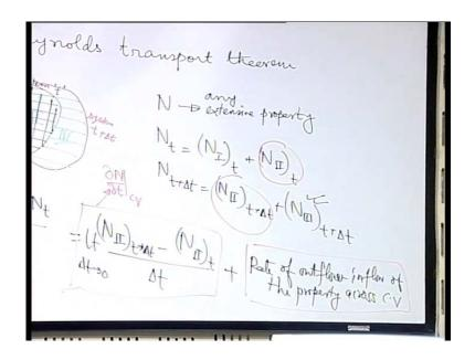
Like, just we can first write this one. This one is nothing but, partial derivative of N with respect to time in the control volume. Because here we are fixing the position and changing N with respect to time, that is why it is the partial derivative.
