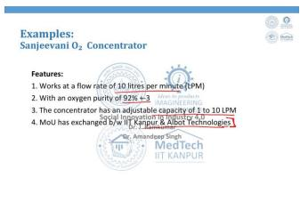
The features of the oxygen concentrator are that it has a capacity of 10 litres per minute, and the oxygen concentrator has a purity of oxygen of around 92% plus minus 3.
